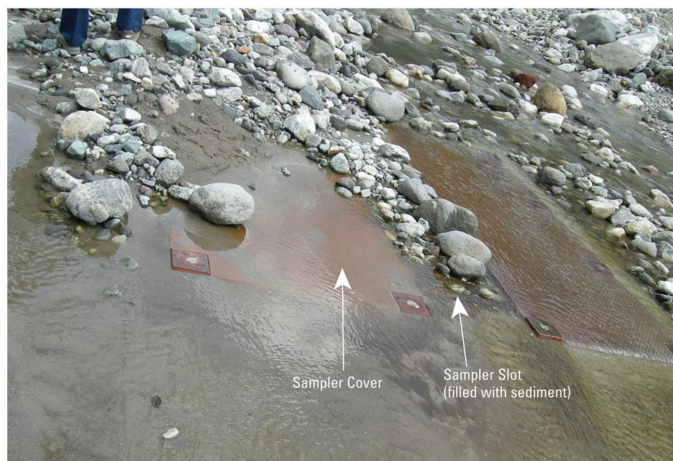
Figure 11. View of a (A) pipe geophone located on a stable bed surface of a slotted debris dam on the Joganzi River, Japan. Flow is from right to left. (B) An automatic, continuously recording Reid-type bedload slot sampler located upstream of the slotted debris dam used to calibrate the pipe geophone. Flow is from lower right to upper center. This is the largest sampler of its kind, with a total volume of 9.25 cubic meters and a slot width of 1 meter. The slot sampler is full of captured bedload following a flood.
