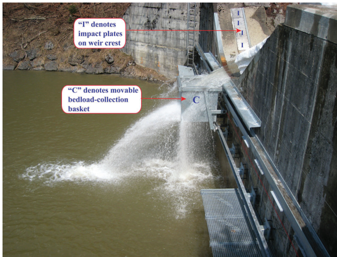
Figure 13. Impact plate array for measuring bedload transport in the Erlenbach stream, Switzerland (lateral view of the tailwater section, with plates visible in the upper right and water falling into an automatically driven basket-type bedload sampler). Sensors are mounted underneath the steel plates at the crest of the large check dam. The moveable bedload-collection basket provides calibration data. Photograph courtesy of Dieter Rickenmann.
