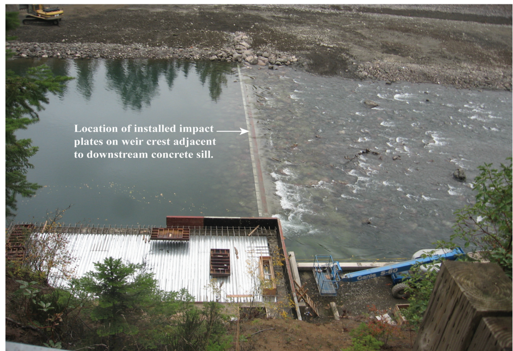
Figure 14. Plate geophones deployed across the Elwha River, Washington, United States; flow is from left to right. (A) Grouted riprap is present upstream and downstream of the weir before removal of the wood retainer to emplace the geophone impact sensors. (B) the operational geophone installation (photograph (B) by Timothy J. Randle, Bureau of Reclamation)
