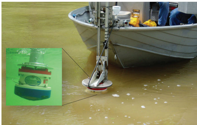
Figure 10. An acoustic Doppler current profiler (ADCP) deployed from a boat (photograph courtesy of Paul R. Baker, USGS), with inset showing a submerged ADCP (photograph courtesy of Timothy J. Reed, USGS).
