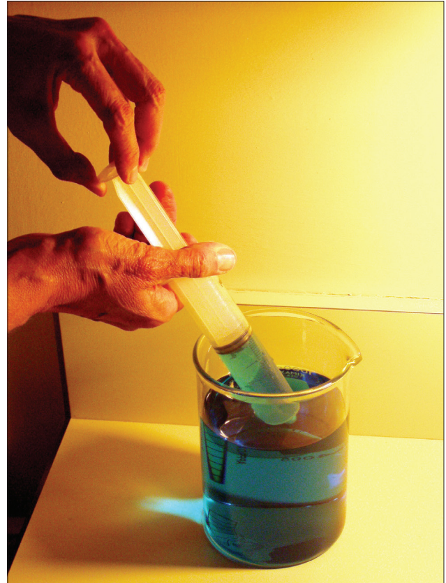
Figure 8. Syringe in a beaker of water, used to illustrate the effect of how a drop in barometric pressure draws soil gases into a structure.
