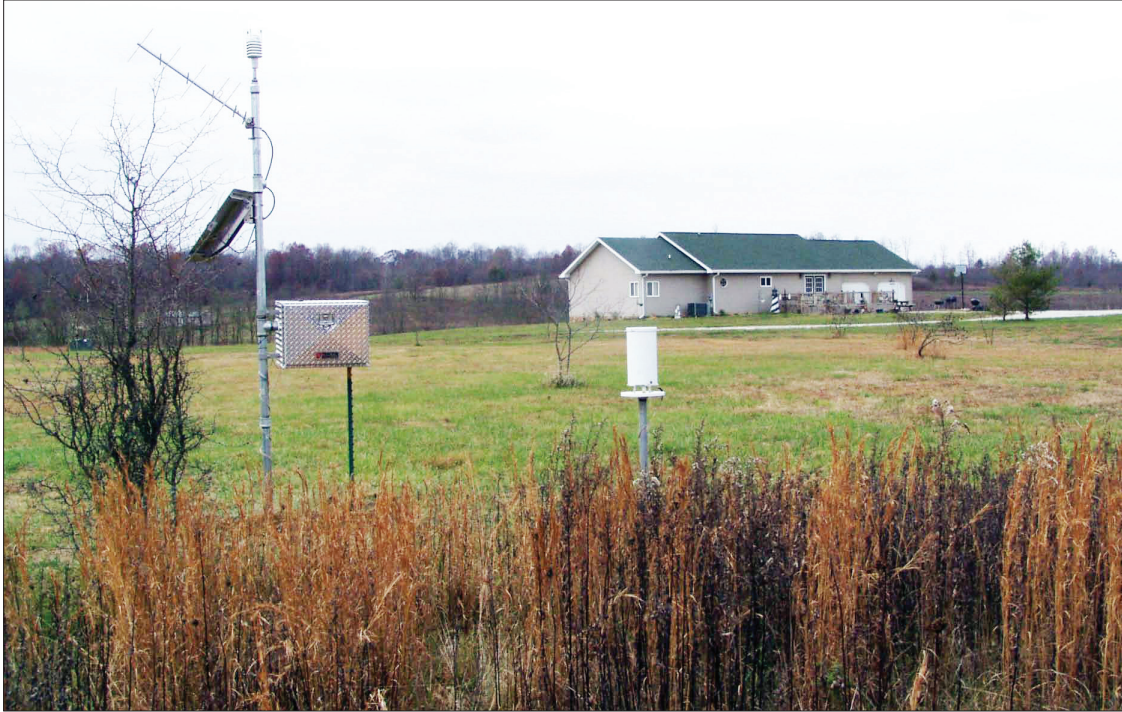
Figure 5. Meteorological observation platform designed for hourly transmission of local meteorological data measured at the Pike County, Ind. study site.
