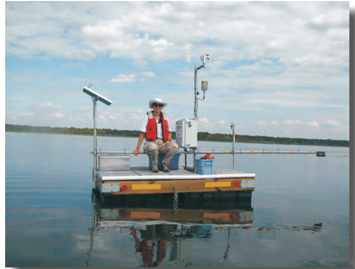
Floating data-collection raft on Lake Panasoffkee, carrying a suite of instrumentation to measure air and water temperature, relative humidity, windspeed, and net radiation; photo by W. Scott McBride
