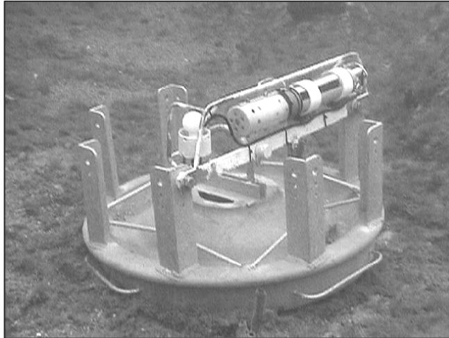
Figure 2.8.2.1. Ocean Sentinel Platform with YSI 6000 Data Sonde and light diffuser installed at the East and West Flower Garden Banks.
