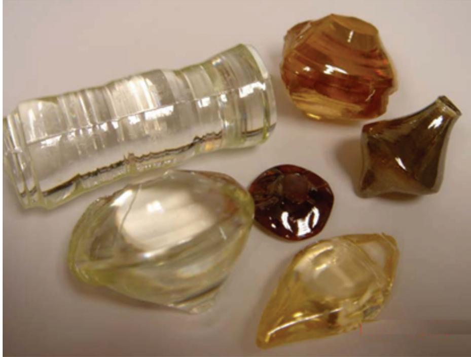
Figure 14. Pure and doped LN crystals grown at AAMU.
