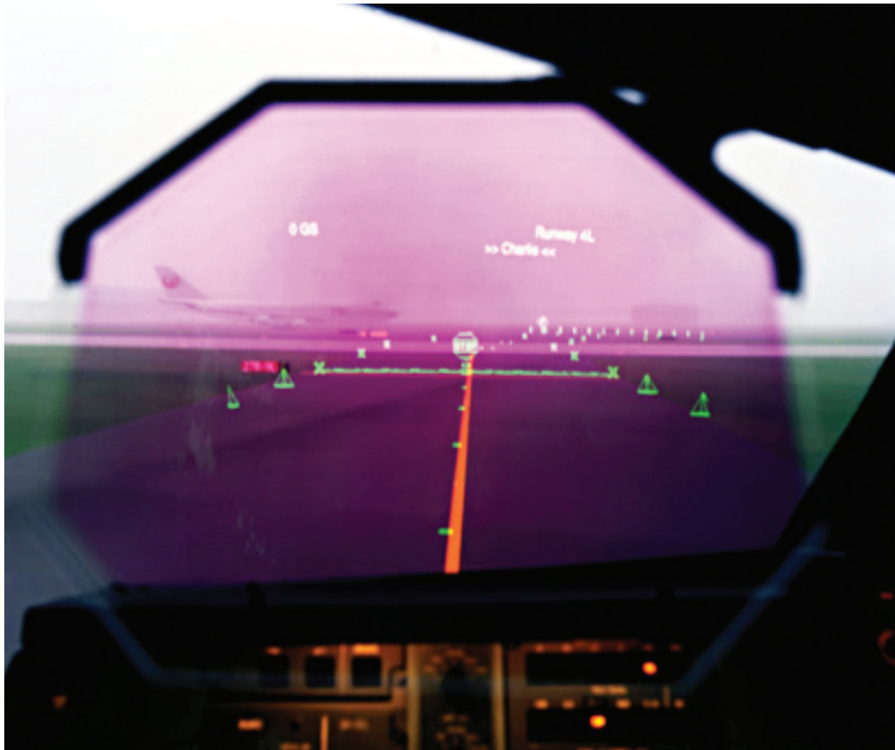
Figure 2: A HUD visualizing a potential runway hazard (NASA Ames Research Center).
