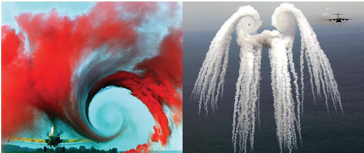
Figure 2: The vortices created by high-lift, low-speed conditions seen on runways (left) and at high subsonic cruising speeds (right) (NASA).
