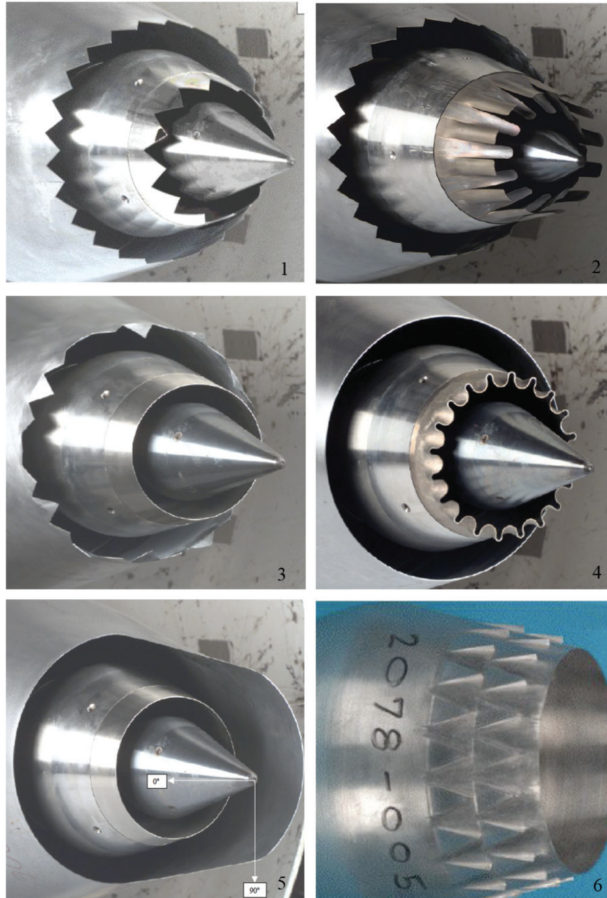
Figure 1b: The above six images show various types of noise-suppression devices from the AST program. From top to bottom, left to right are (1) fan and core chevron nozzles, (2) the core tongue nozzle, (3) the tabbed fan nozzle, (4) the core lobe nozzle, (5) the scarfed fan nozzle, and (6) the vortex doublet core nozzle (NASA/CR 2000-210040).
