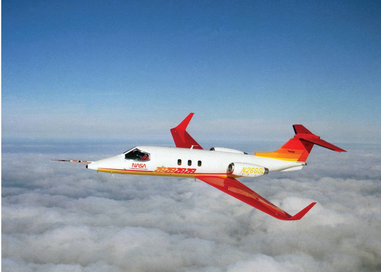
Figure 5: The Learjet Model 28 with its newly designed winglets (NASA Langley Research Center, UID: SPD-NIX-EL-1997-00215).
