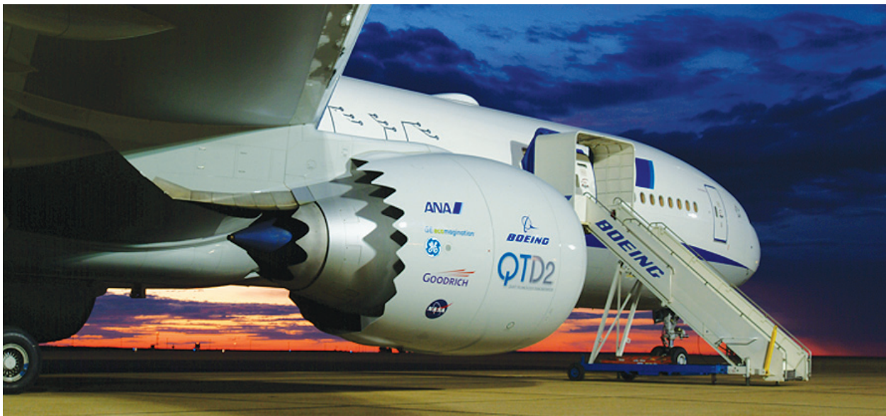
Figure 2b: Azimuthally varying chevrons used in QTD2 program (NASA).
