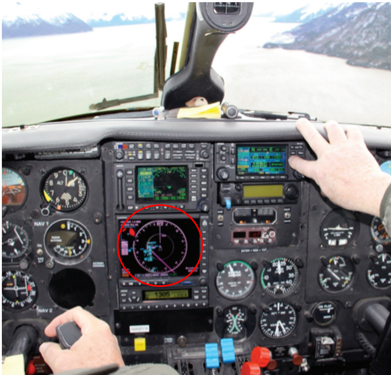
Figure 2: A cockpit fitted with new ADS-B technology (ADS-B Technologies).
