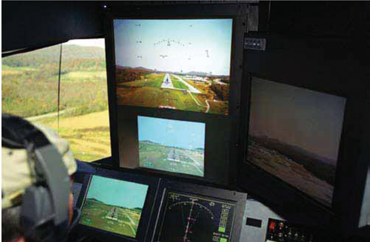
Figure 3: Simulated cockpit view using external vision systems (XVS) technology (NASA High Speed Research program).
