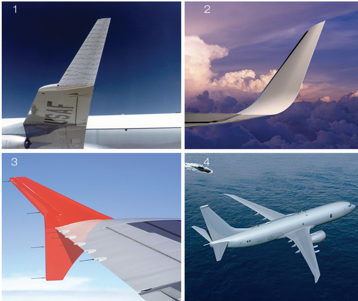
Figure 6: Various wingtip devices in use today are shown here, including the (1) “traditional” winglet, (2) blended winglet, (3) wingtip fence, and (4) raked wingtips ([1] NASA Dryden Flight Research Center, UID: SPD-NIX-EC79-11481; [2] Aviation Partners, Inc.; [3] Bruce Leibowitz, Northwest Airbus A319, N353NB, Sept. 2003; [4] The Boeing Company, DVD-1147-1, copyright 2005).
