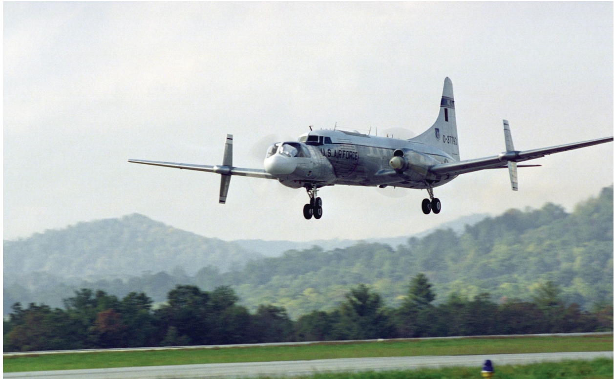
Figure 5: The TIFS dual-cockpit research airplane (NASA Image EL-199-00568).
