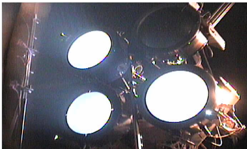
Figure 2.—"3+1" configuration NEXT multi-thruster array operating in Vacuum Facility 6 at NASA GRC. Faraday probe rake is visible on the left.
