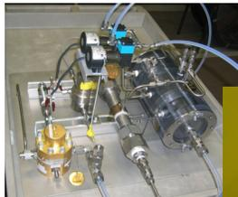
**Integrated Ejector/Regulator and Integrated Ejector/Regulator/Two-Stage Water Separator System**
