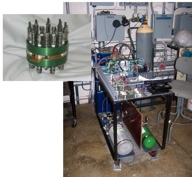
Shown: Infinity Lab Stack #3 and test rig with fuel cell system (stack + balance-of-plant)
