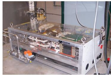
Teledyne multi-kW flow-through PEMFC Breadboard
