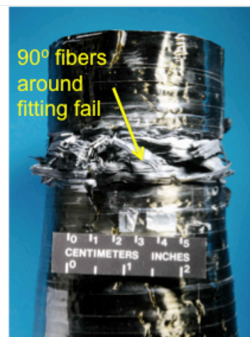
Fig. 30. Failure of a corrugated fitting strut.
