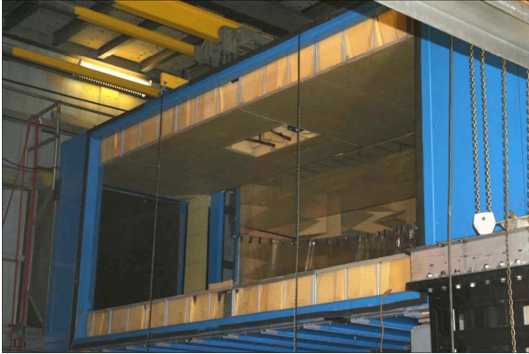
Figure 4. Exterior view of the anechoic test section with the acoustic windows and the port side anechoic chamber removed; starboard-side anechoic chamber visible in the background
