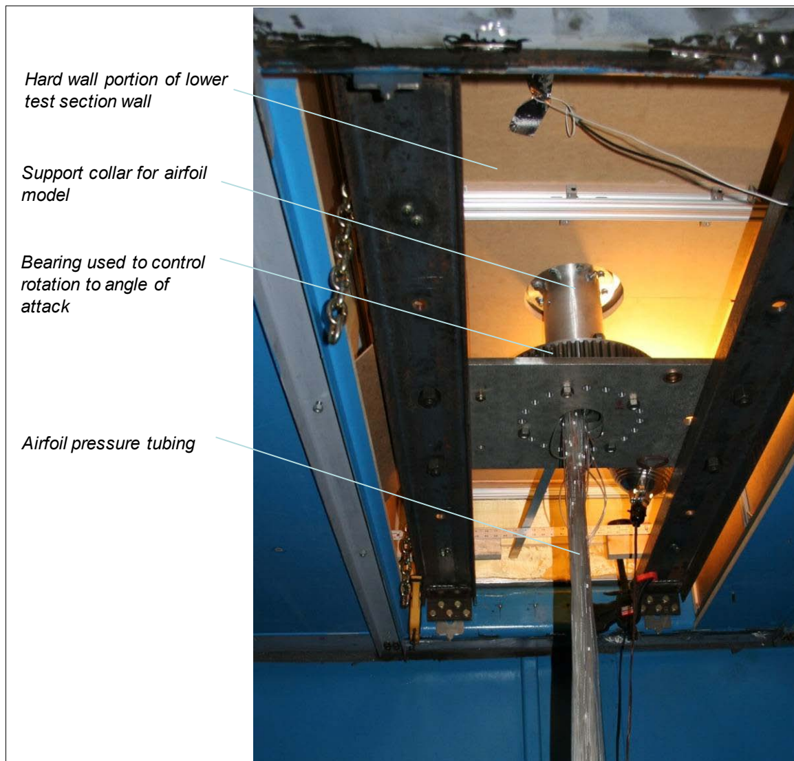
Figure 9. Photo matching Figure 5, but taken from beneath the test section showing the collar and bearing arrangement that form the airfoil-mount bearing arrangement
