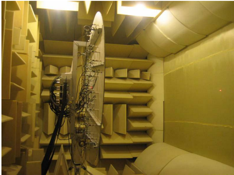
Figure 19. Microphone arrays used in the two test entries (a) star array and (b) equal-aperture spiral array
