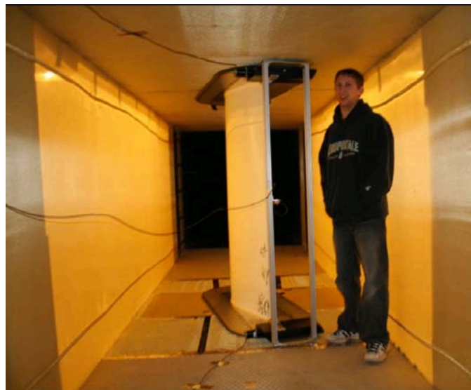
Figure 7. Airfoil model mounted in the test section as configured for the November-December 2007 entry, as seen from downstream (note the end plates on airfoil model and the partially installed trailing-edge hot-wire traverse)
