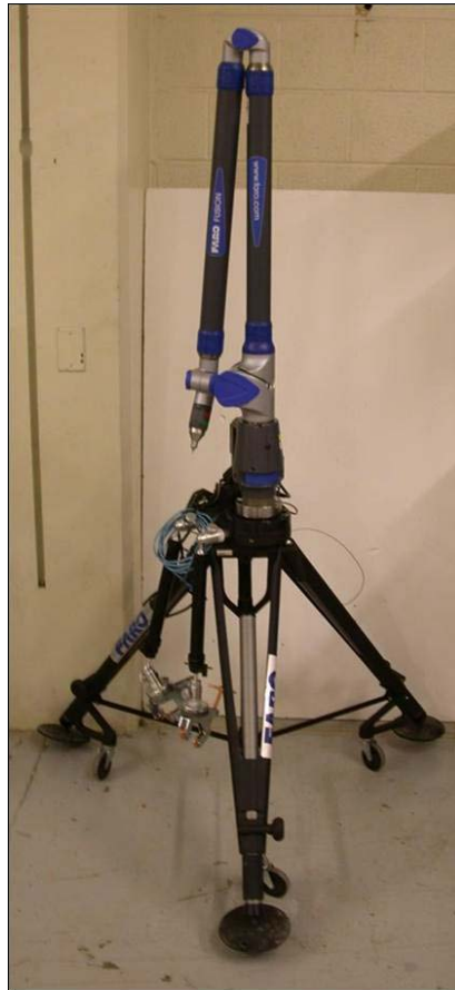
Figure 199. FARO Fusion Arm CMM used for measuring the manufactured wing models
