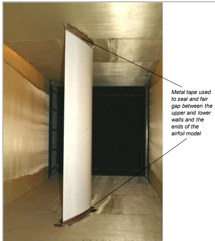
Figure 6. Airfoil model mounted in the test section as configured for the July 2007 entry, as seen from downstream; identical support and panel arrangements are used on the lower and upper walls
