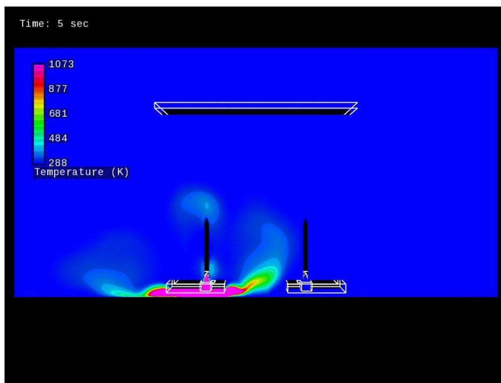
Figure 7.5-9. Temperature of Exhaust Plumes 5 seconds After Ignition of Boosters in High Bay 3 in the Cut Plane Between High Bays 3 and 4 During Scenario 1d
