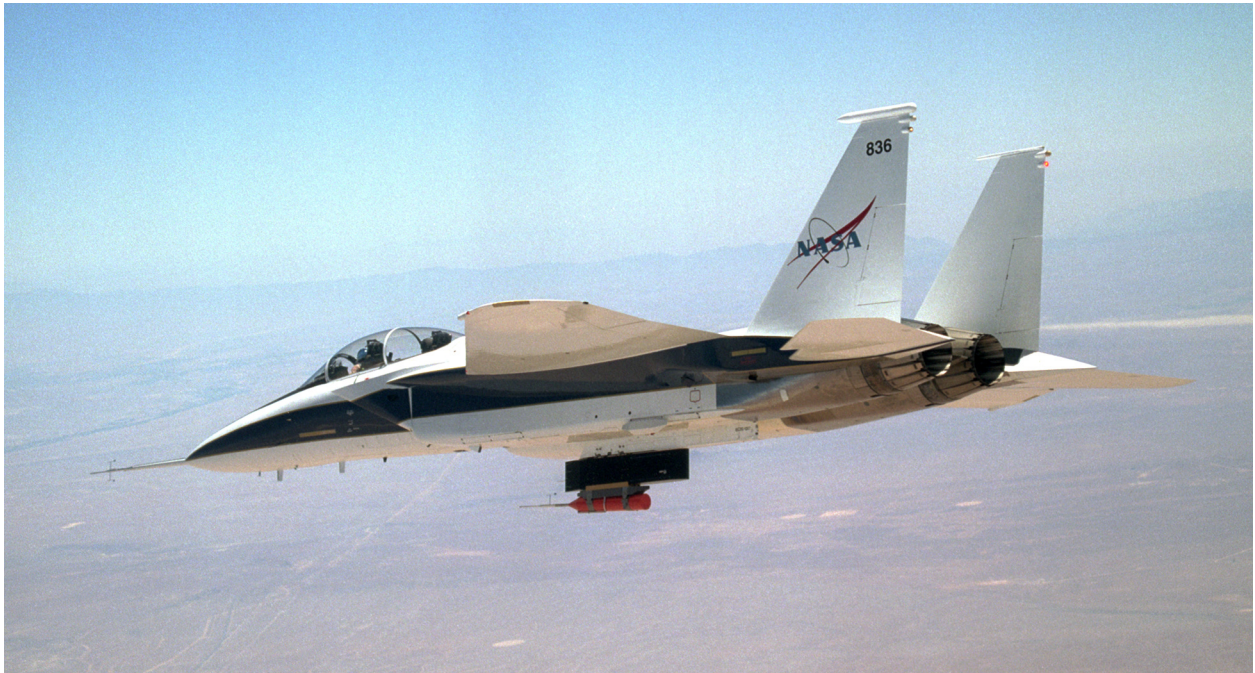
Figure 1. The NASA F-15B airplane with the Propulsion Flight Test Fixture local flow experiment, in flight.
