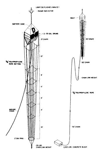
Figure 1.--Fish aggregating device, buoy type.
