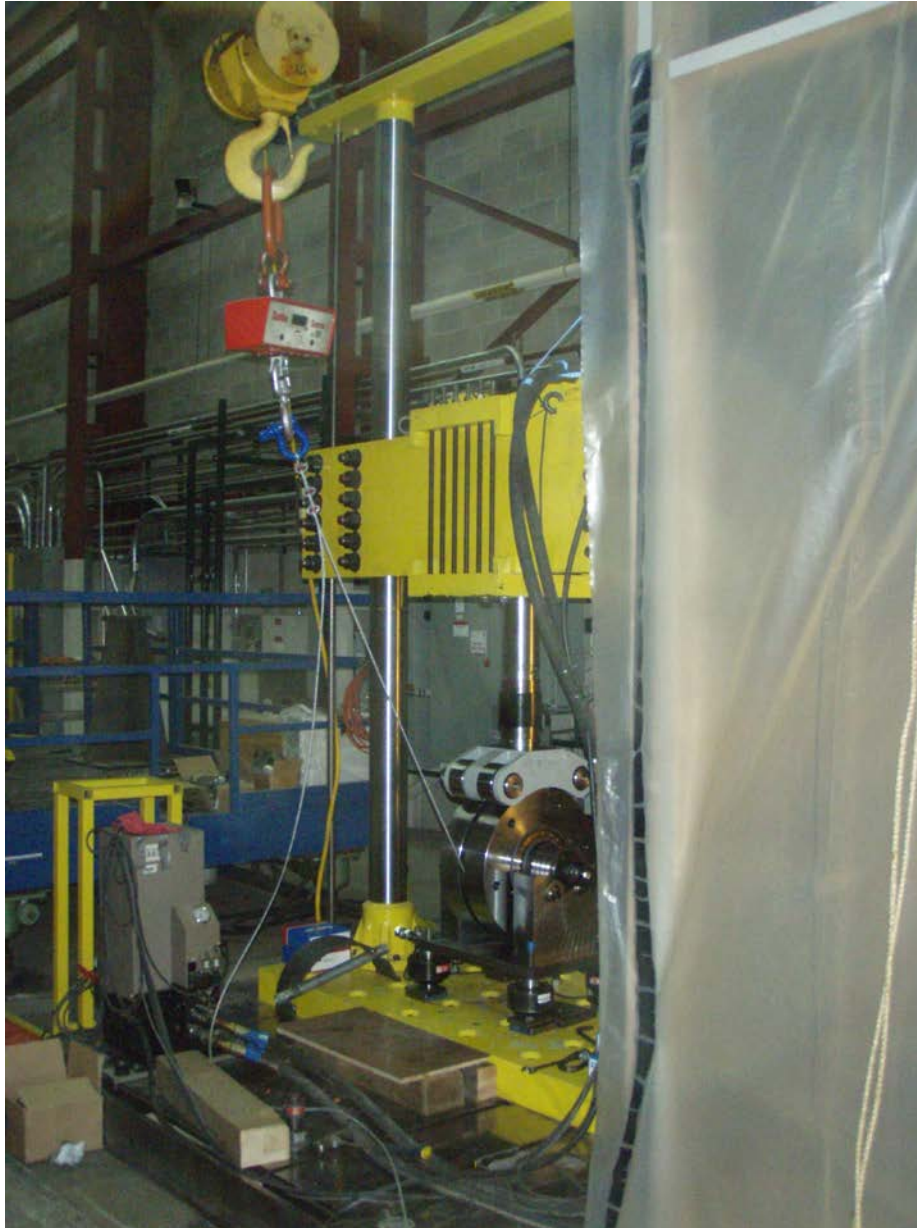
Figure 11. Crane calibration method set up. PIX #19677.
