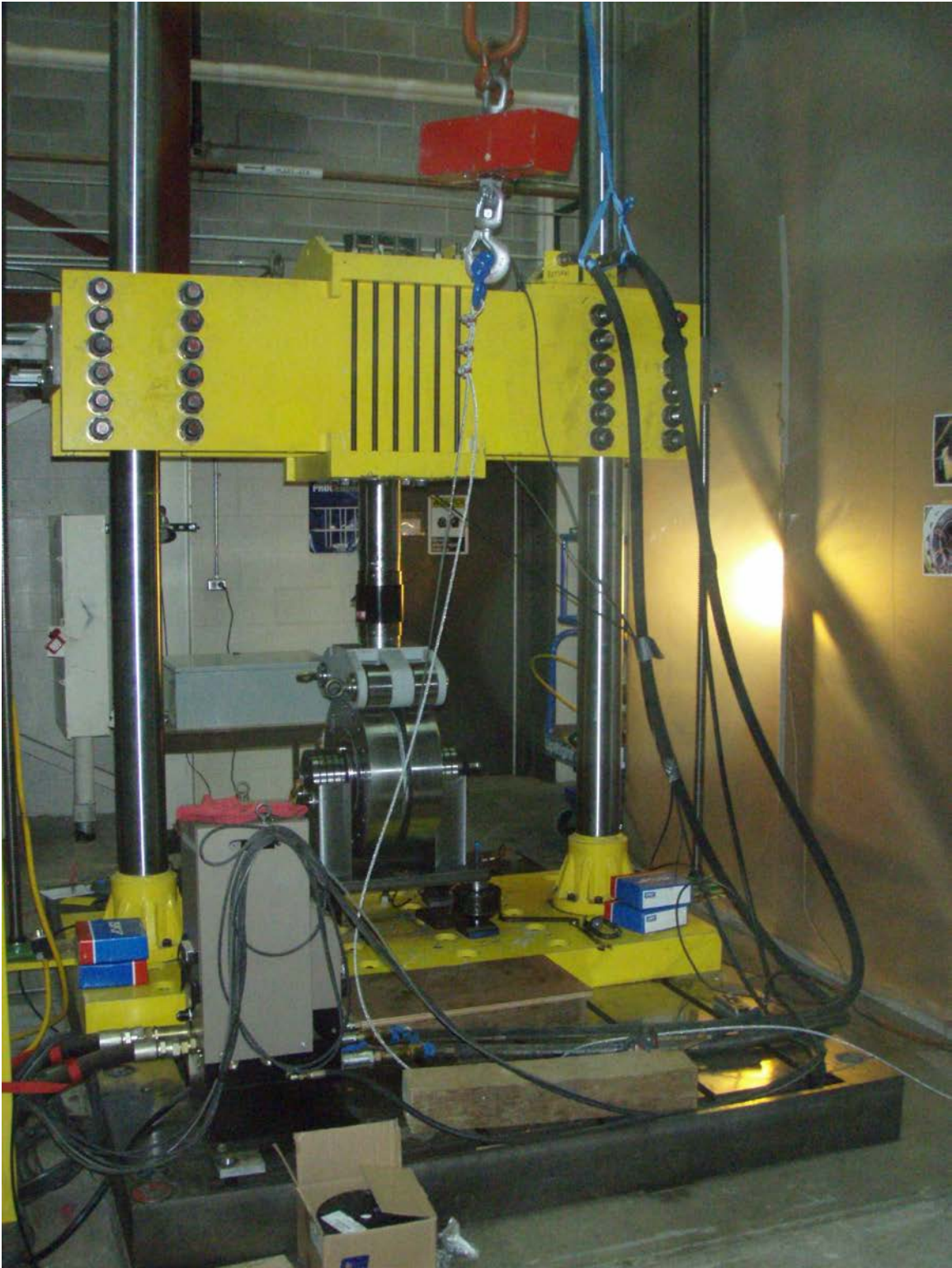
Figure 6. Calibration stand in the 100 kip load frame in the 251 highbay. PIX #19676.
