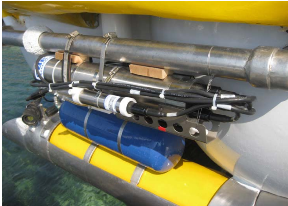
Figure 5. A Seabird Seacat 19 CTD-O water chemistry profiler mounted on the starboard rail.
