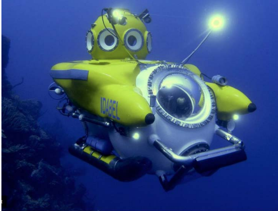
Figure 3. Idabel submersible is a three-person sub with a 32in. (81 cm) viewport for scientific observers.
