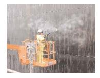
Surface washing agents also are used to clean and decontaminate response equipment and, less often, vessels that have been oiled. For example, in 2001, the M/V Genmar Hector (left) was cleaned with surface washing
