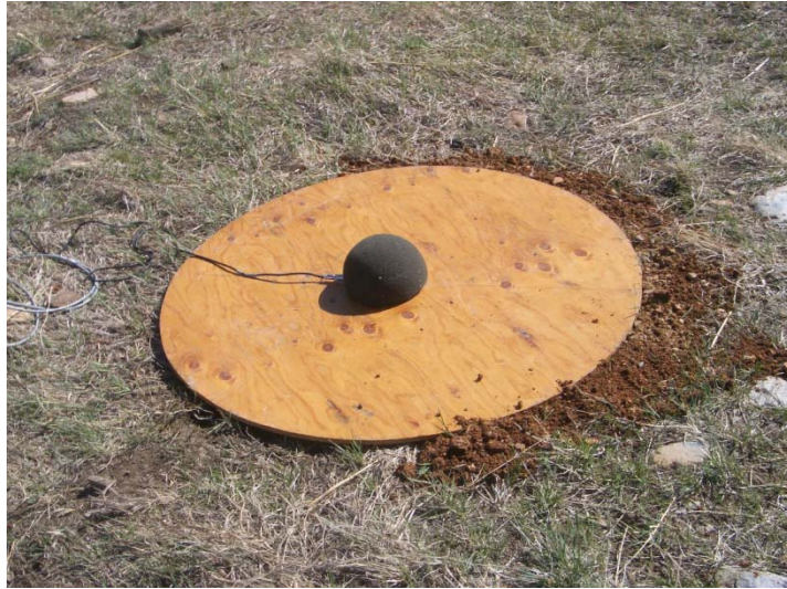
Figure 6. Picture of sound board during the test. PIX #19420.
