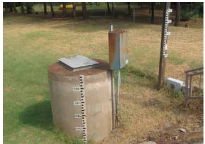
Figure 2. Staff gage operated by the City of Wichita Falls, Texas (photograph courtesy of Davis Powell, City of Wichita Falls).
