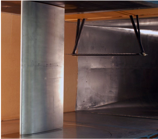
Figure 7.—Subscale NACA 23012 aerodynamic model installed in the University of Illinois wind-tunnel test section.
