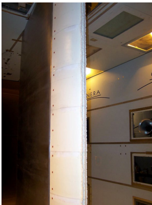
Figure 23.—Completed installation of EG1164 horn ice-shape casting sections on the leading edge of the NACA 23012 airfoil model (upper surface view).
