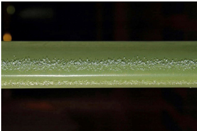
Figure 2.—Photograph of subscale model ED0762 roughness shape. (No tracing was made for this shape.)
