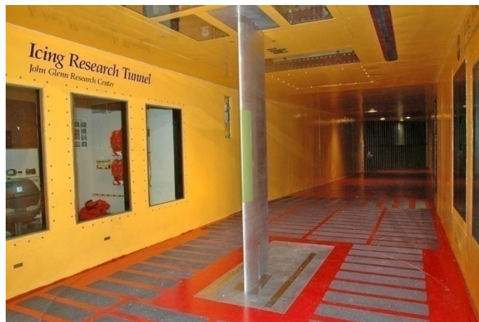
Figure 1.—Subscale NACA 23012 ice-accretion model installed in the NASA Icing Research Tunnel.
