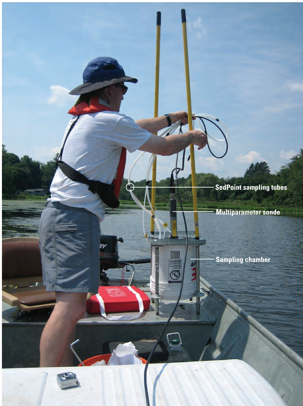
Figure 19. U.S. Geological Survey personnel preparing to deploy the sediment-phosphorus flux chamber.
