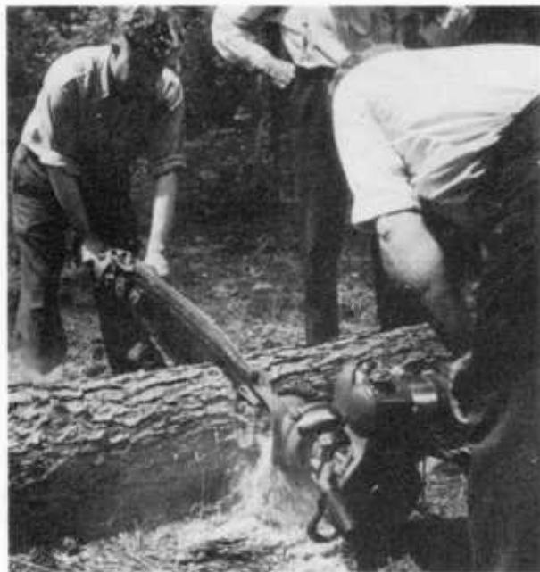
Figure 83.—The operator at the motor end rests his load on the ground whenever possible.
