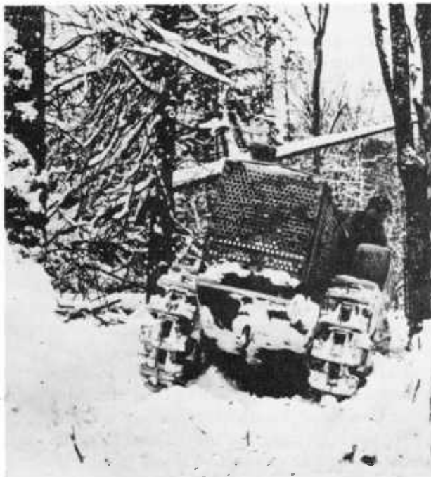
Figure 198.—Skeleton-track shoes are helpful in snow. (Courtesy of Caterpillar Tractor Co.)
