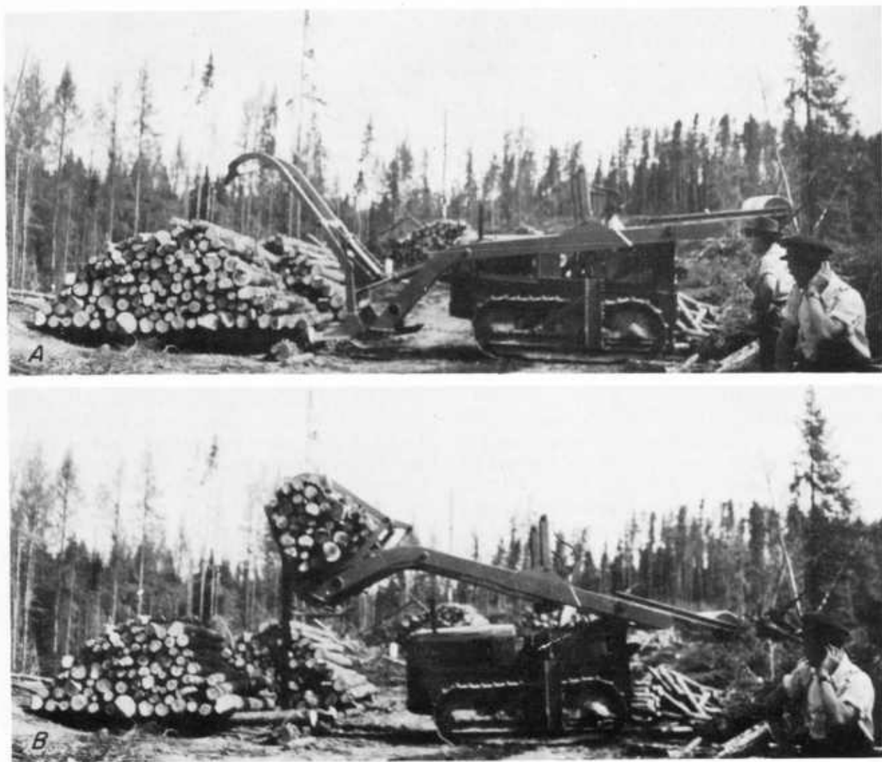
Figure 265.—The skid loader: A, Pushing its arms into a pile of wood; B, picking up an armful.
