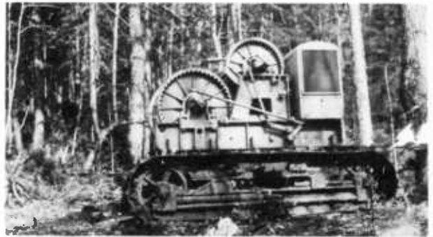
Figure 255.—Double-drum winch mounted on tractor tracks.
