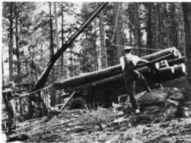
Figure 287.—Loading with crotch line and end dogs.
