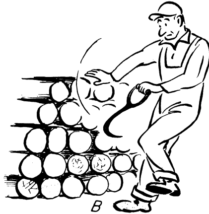
Figure 105.— The safe way, A, is to book the end of the stick, not the side, B, where book may glance off.
