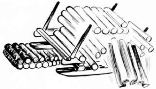
Figure 268. — A ramp for tilting a load off a sled.
