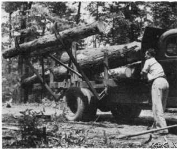
Figure 284.—The “log flipper”. Logs are rolled into the cradle formed by the two arms, then they are flipped over the stakes into the truck.
