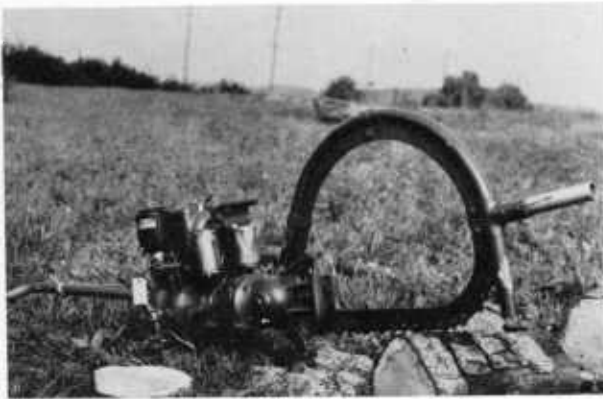
Figure 72.— A bow-type chain saw.
