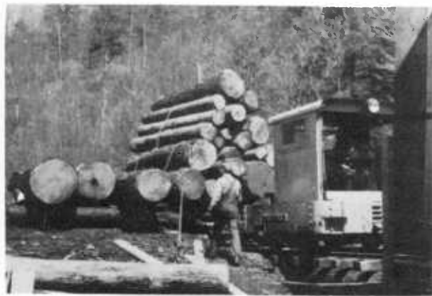
Figure 334.—Small locomotives are reviving an interest in tramways. This is a diesel engine.
