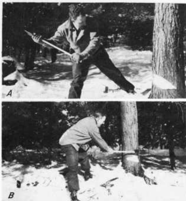
Figure 19.—Stance for chopping. A, Top of ax stroke. Notice position of hands. B, End of ax stroke. The upper hand has slid down the handle.
