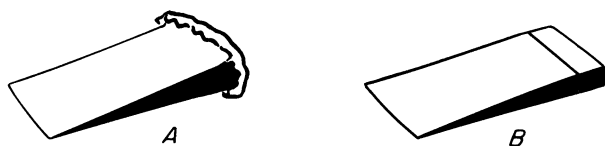
Figure 86.—A mushroomed head, A, should be ground off. B, Wedge after grinding.
