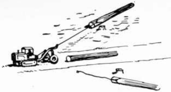
Figure 214.—Bunching logs at a roadway.
