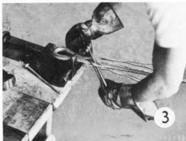
Figure 234.—Steps in splicing an eye loop: Step 1, the thimble and wire are clamped in a rigger's vise. Step 2, the short end is unlaied. Step 3, strands are inserted and tightened with marlinspike. Step 4, completed splice ready for wrapping.
