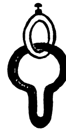
Figure 175.—The jews-harp ring holds a chain well at any link.
