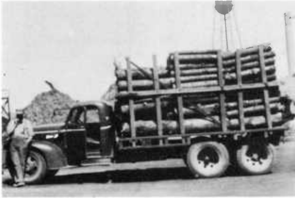
Figure 338.—Truck with side racks for carrying pulpwood.
