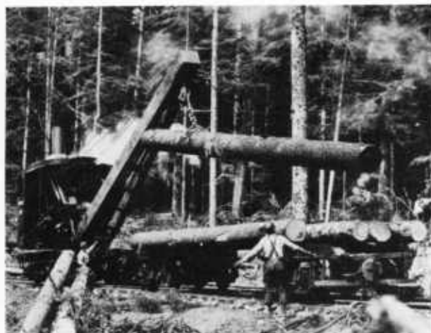
Figure 290.—With a heel boom the log can be placed safely and accurately.
