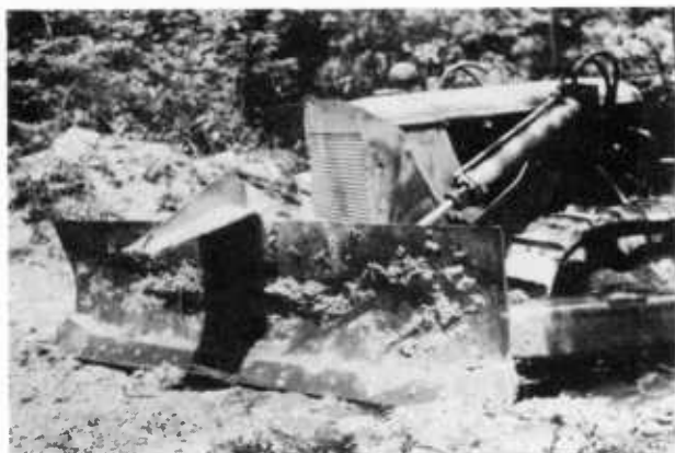
Figure 320.—A pusher bar is welded on this dozer blade.
