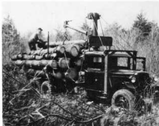
Figure 283.—A home-made jib boom mounted on truck.
