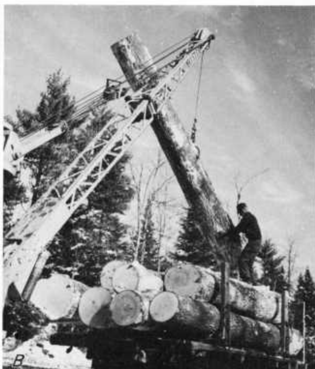
Figure 289.—When tongs are used, the top loader has to catch one end (A) and guide it into position (B).
