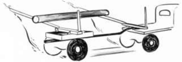
Figure 271.—Skids used in loading from a slope.
