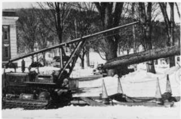
Figure 208.—A log loader and scoot combination. (Courtesy of Arthur Witherell.)
