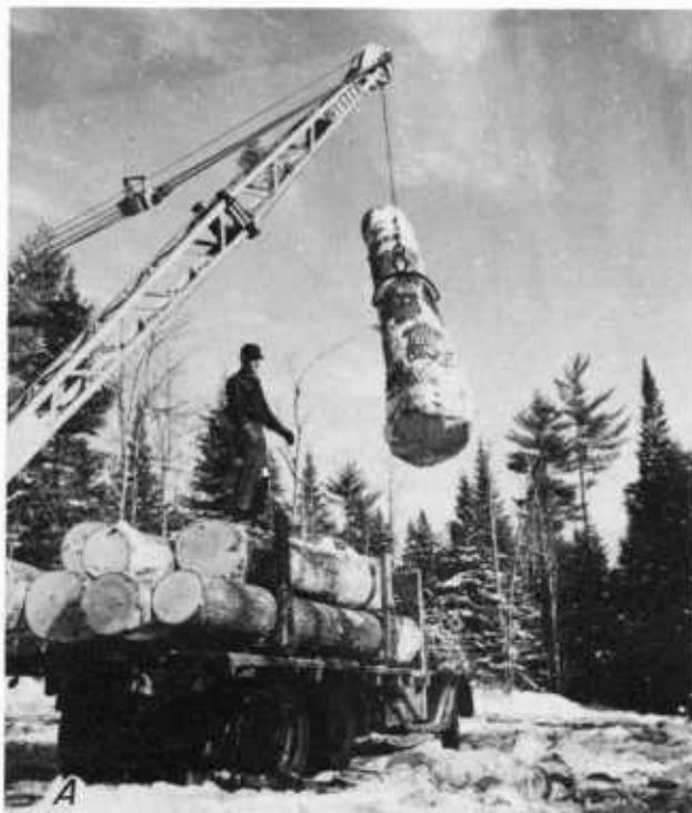
Figure 289.—When tongs are used, the top loader has to catch one end (A) and guide it into position (B).
