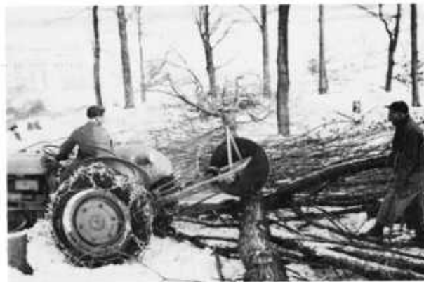
Figure 67.— Circular saw mounted on tractor. (Courtesy of Patch Wegner Co.)
