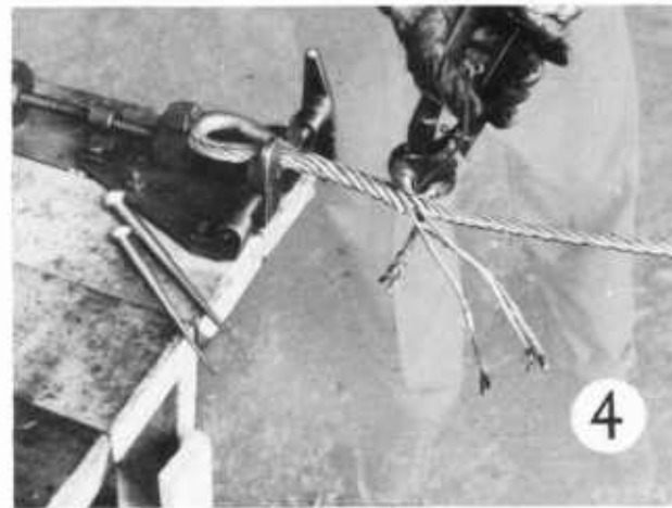
Figure 234.—Steps in splicing an eye loop: Step 1, the thimble and wire are clamped in a rigger's vise. Step 2, the short end is unlaied. Step 3, strands are inserted and tightened with marlinspike. Step 4, completed splice ready for wrapping.
