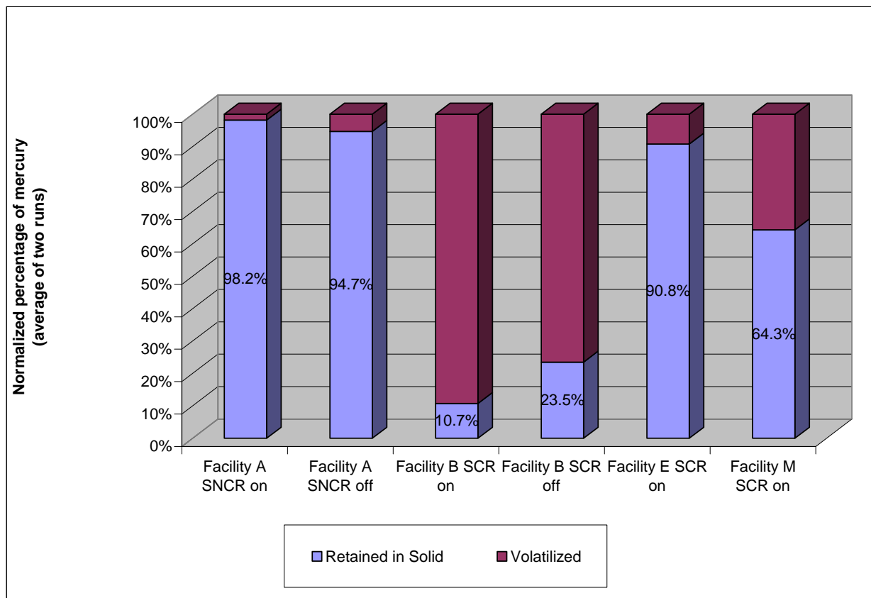
Figure E-4. Normalized results of asphalt simulation tests for non-ADA fly ashes
