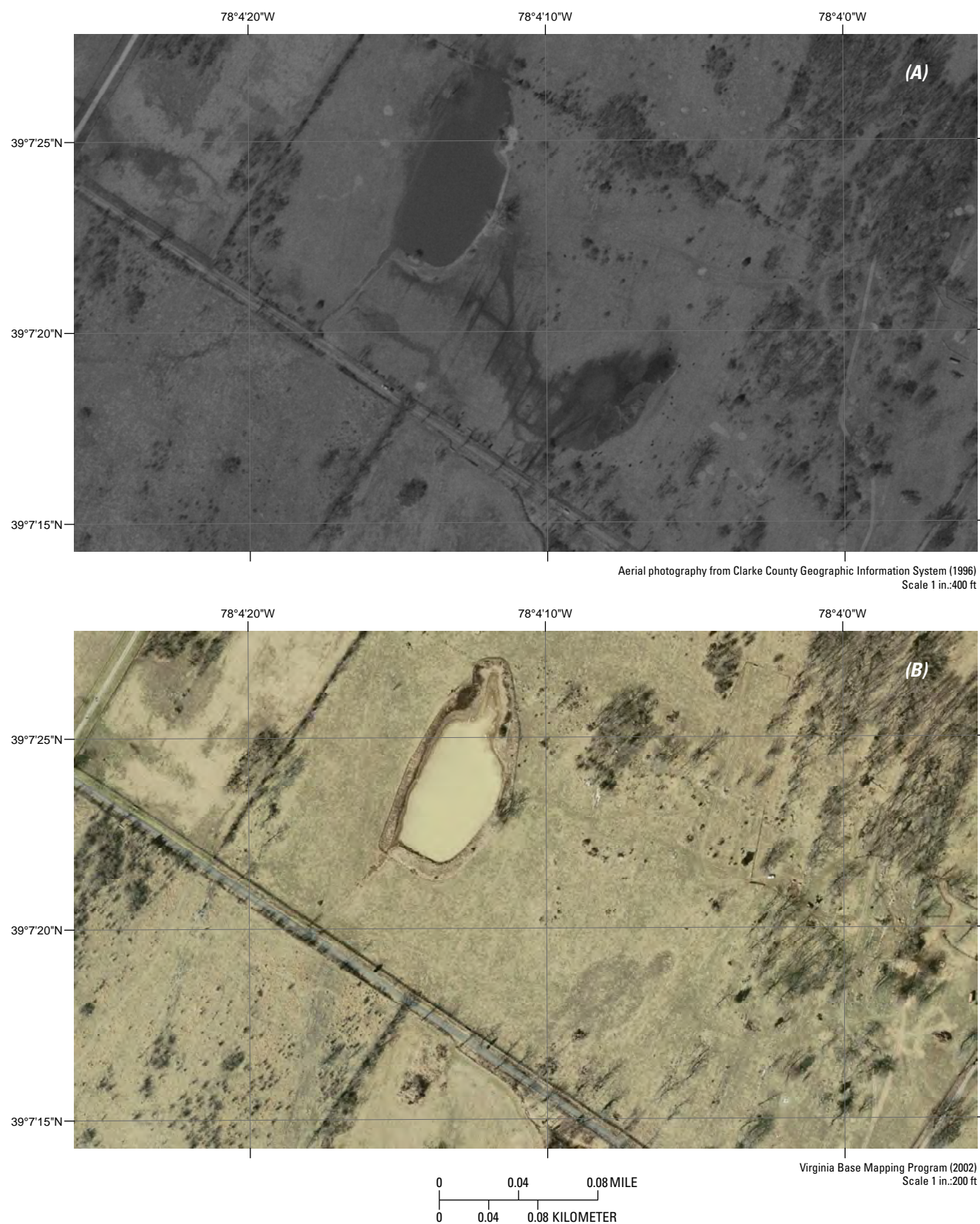
Figure 34. (A) Wet and (B) drought conditions in 1996 and 2002, respectively, for an area along Route 620 in Clarke County, Virginia, where groundwater overflows along bedding and joints (darker tones) in the carbonate rock during wet periods. Strike of the bedding is in northeast-southwest direction.
