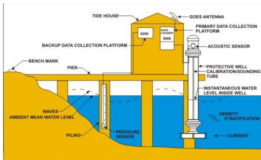
**Figure 3.2.** Schematic of a modern water level station
