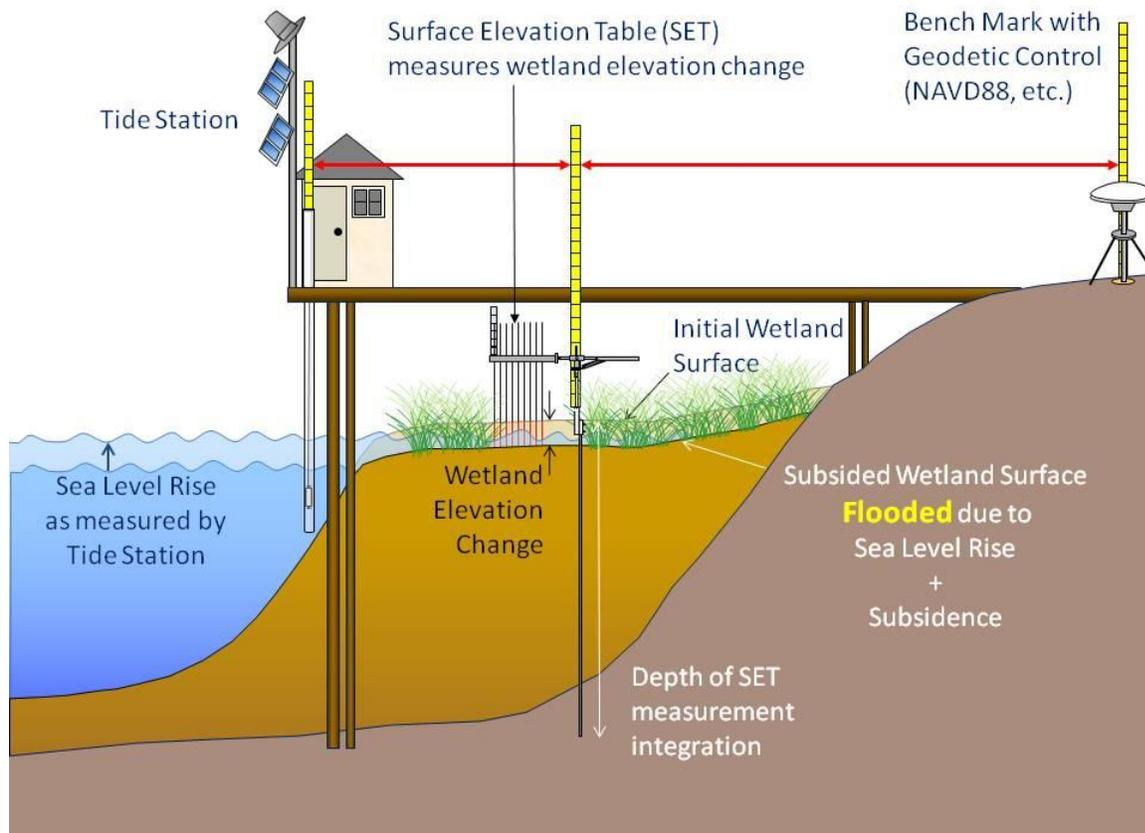
**Figure 3.8.** This conceptual diagram shows how geodetic connections between local tide stations, SETs, and geodetic control can provide a measurement of wetland elevation dynamics relative to locally-expressed (e.g. “relative”) sea level change.
