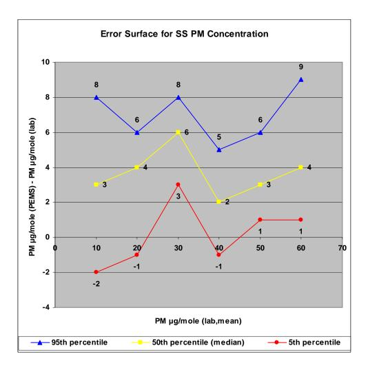
FIGURE 6. ERROR SURFACE: (PEMS-LAB) VS. LAB
