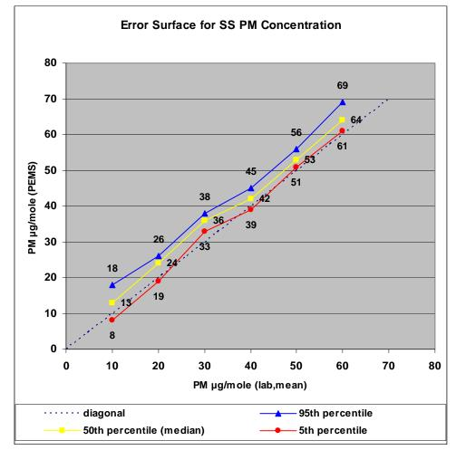
FIGURE 5. ERROR SURFACE: PEMS VS. LAB
