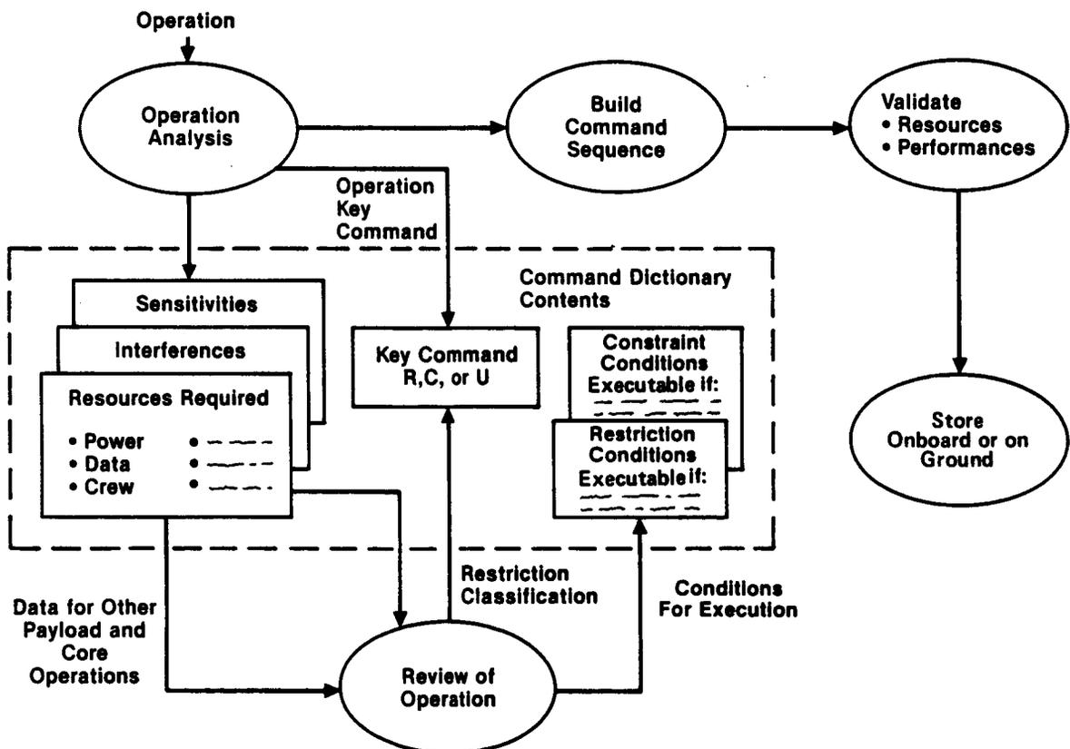
Figure 4-14. Customer Operation Commands Sequence Development
