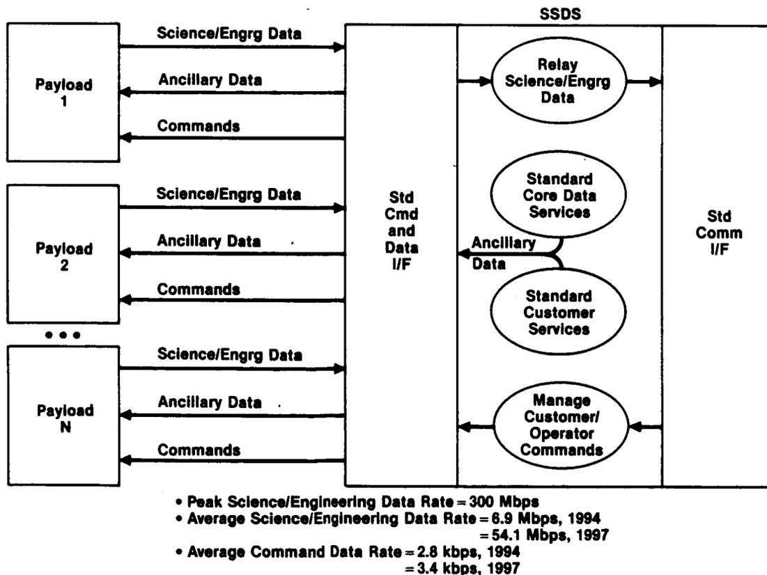
Figure 5-3. SSDS/Payload Data Interfaces
