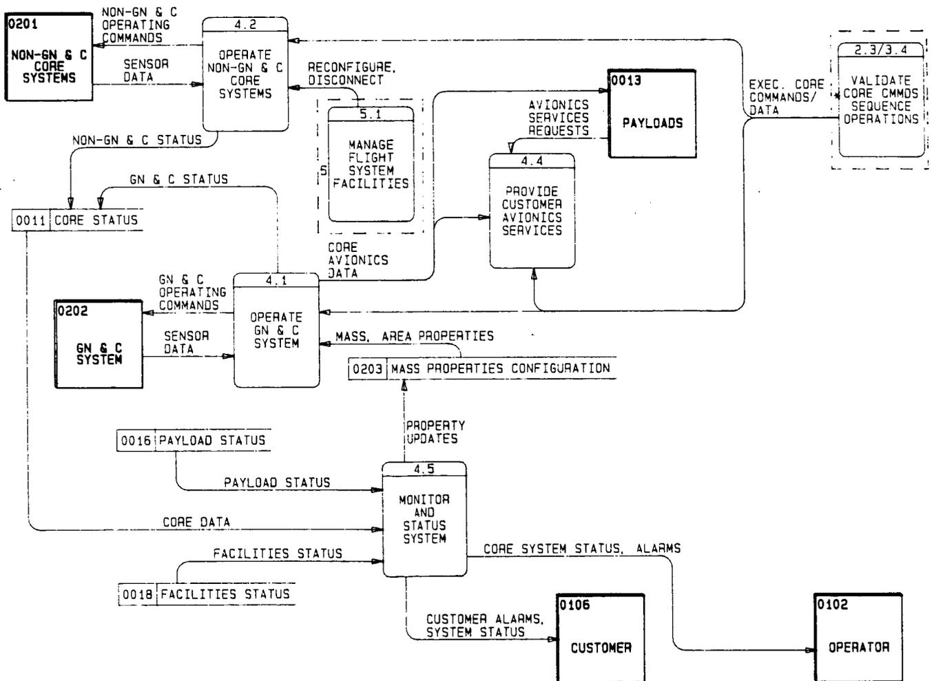
Figure 6-11. SSDS Level 1 DFD - Platforms, 4.0 Operate Core Systems
