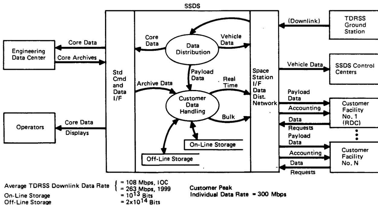
Figure 5-7. Data Network – SSDS Data Interfaces
