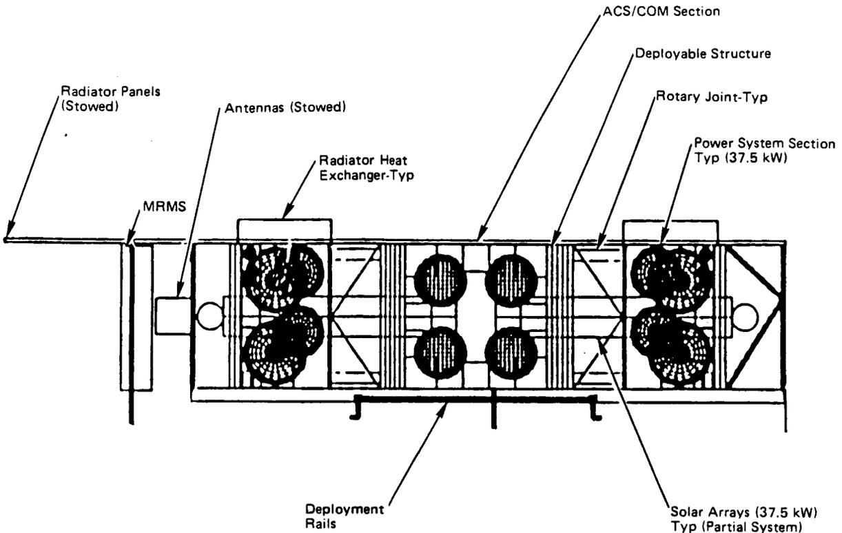
Figure 4-34. Transverse Boom Launch Package-
