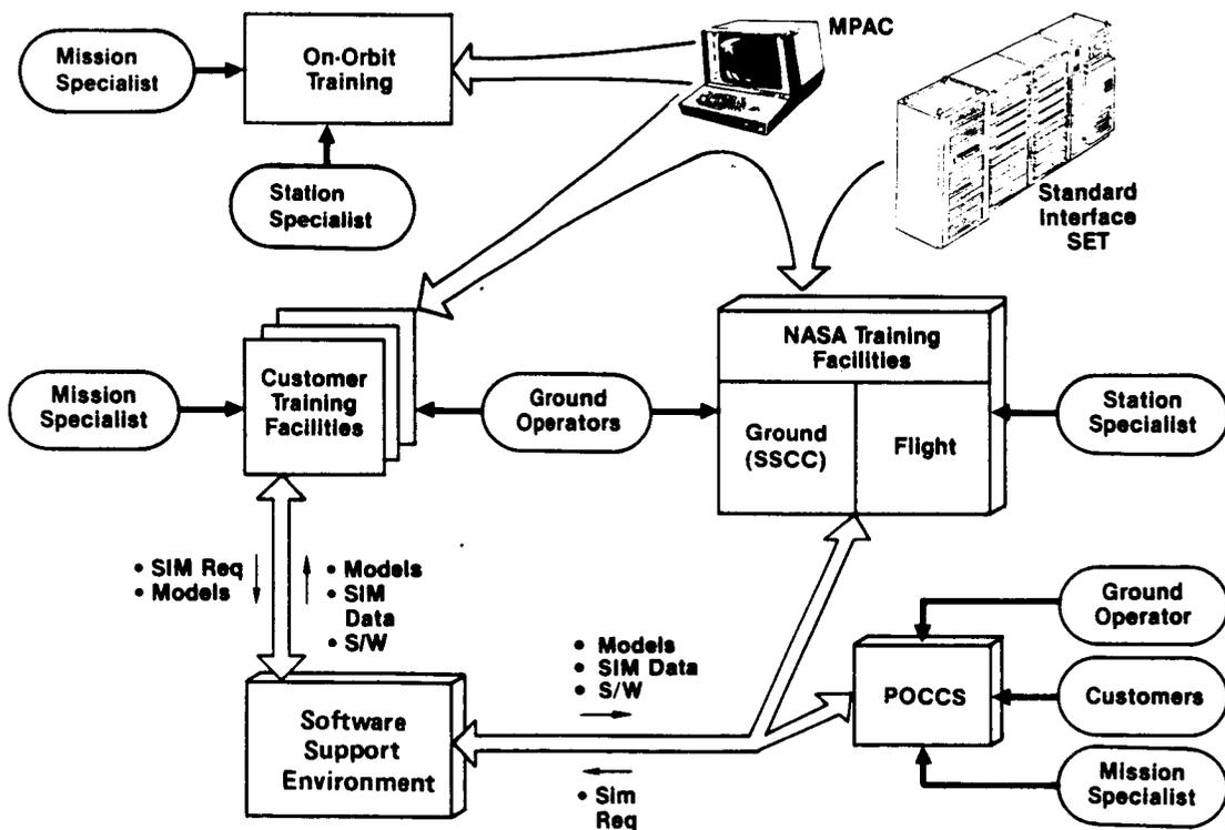
Figure 4-30. Training and Simulation Maximizes Use of Program Operational Capabilities
