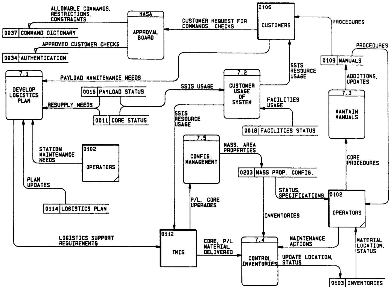
Figure 6-8. SSDS Level 1 DFD 7.0 Support Space Station Program
