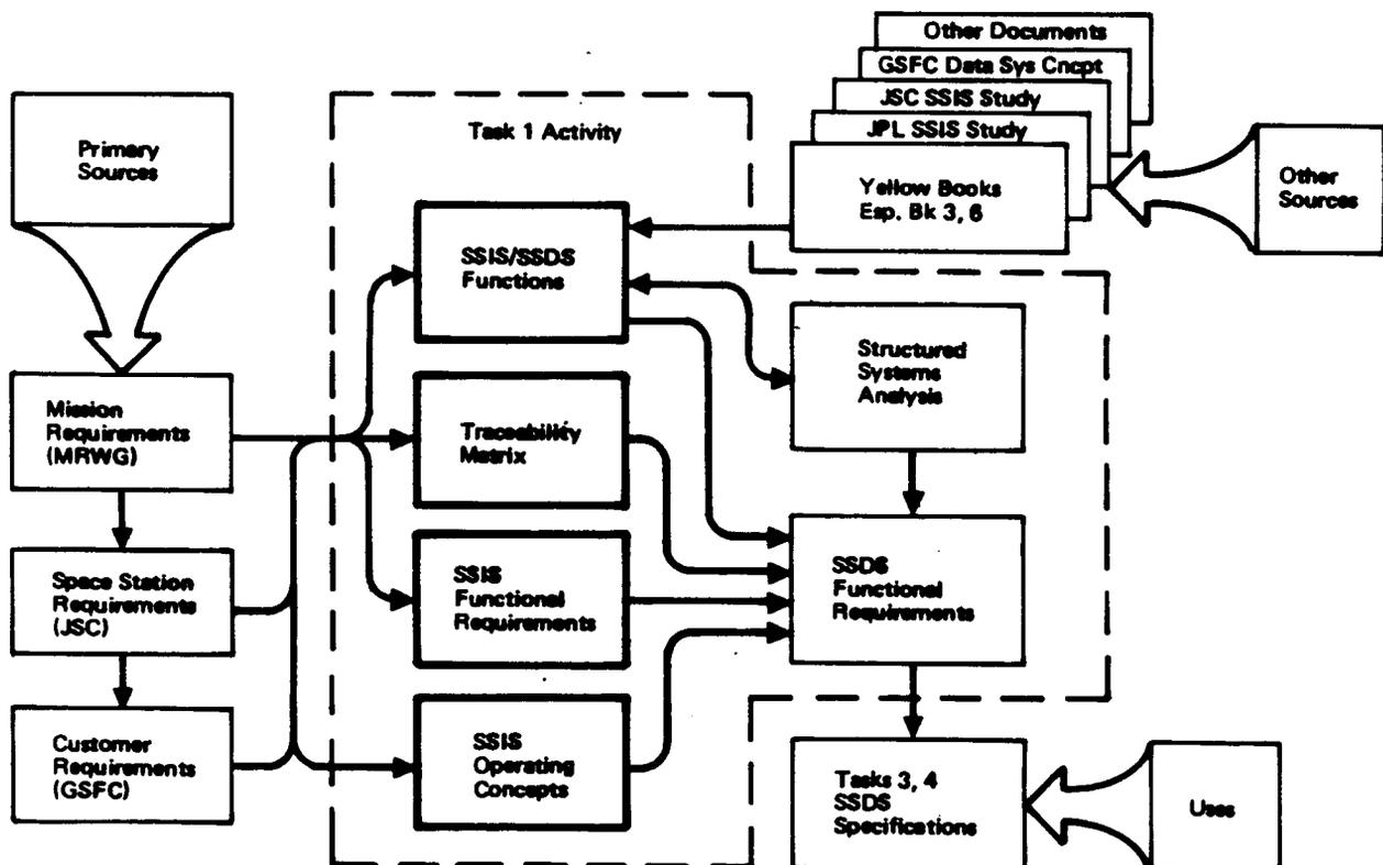
Figure 1-1. Requirements Development Methodology Flow
