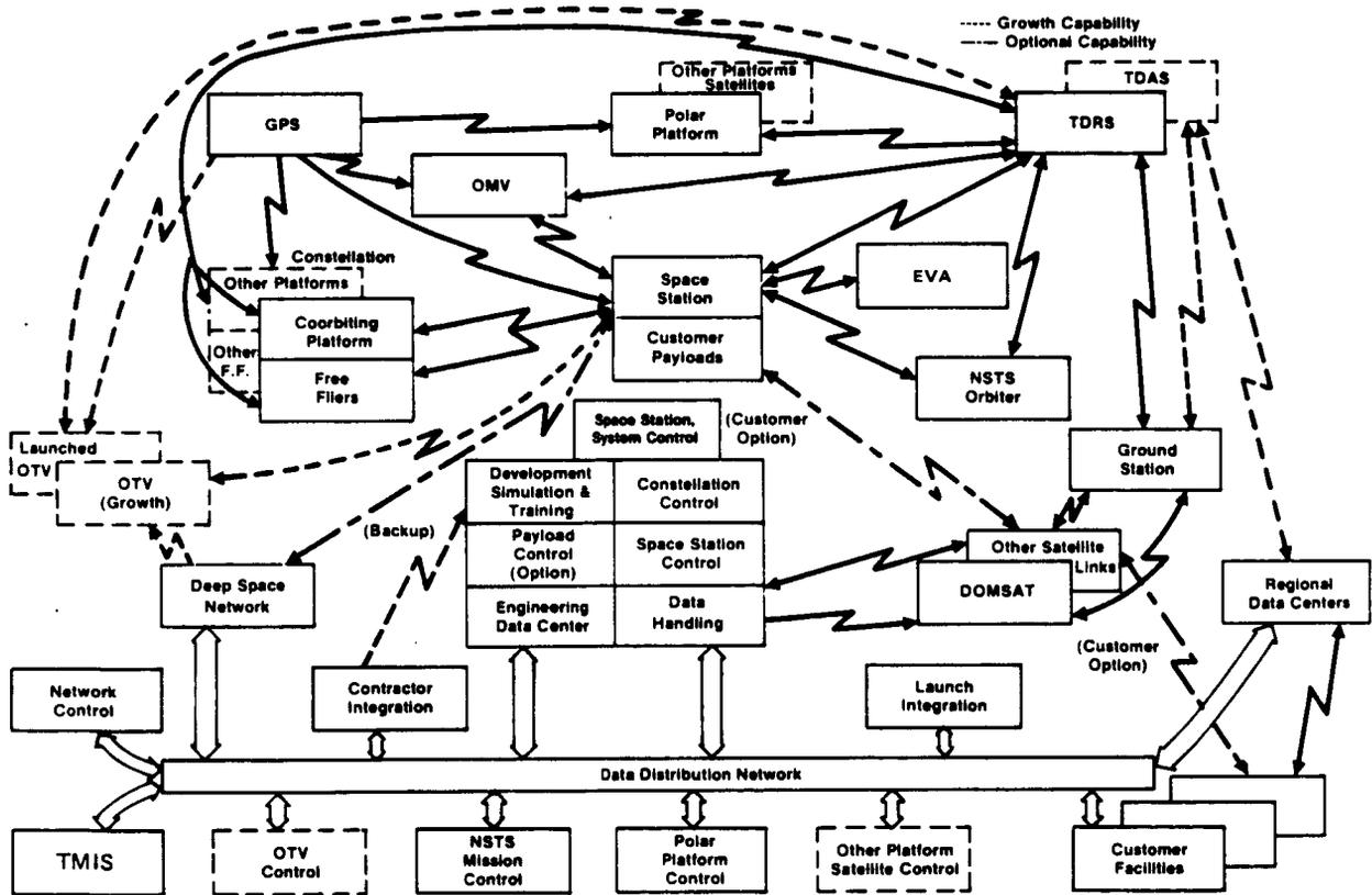
Figure 4-1. Space Station Program Element Interconnection
