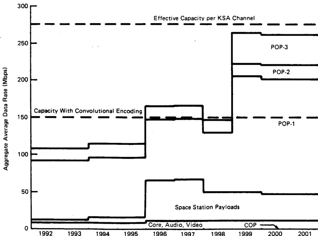
Figure 5-8. TDRSS KSA Channel Requirements Versus Capacity
