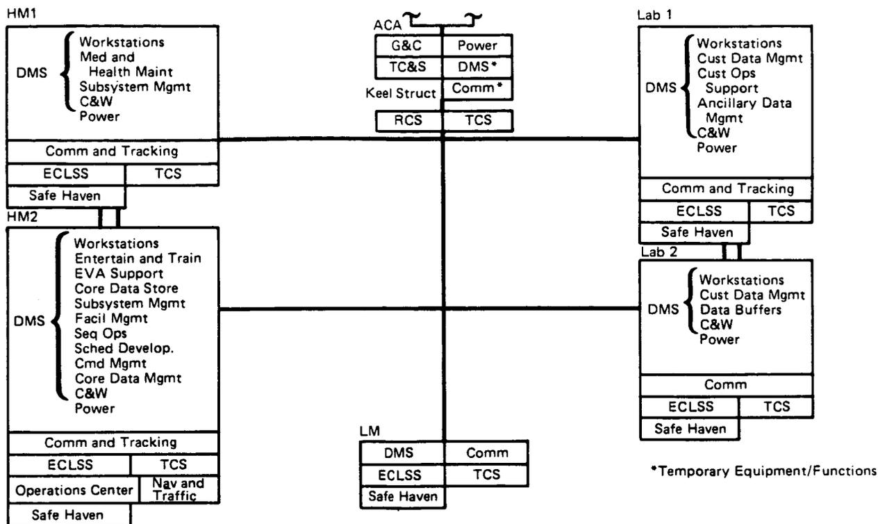
Figure 4-32. Preliminary Space Station Functional Distribution
