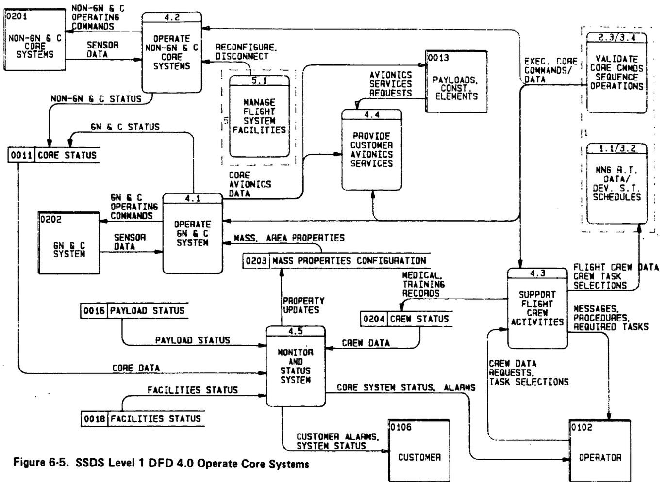
Figure 6-5. SSDS Level 1 DFD 4.0 Operate Core Systems
