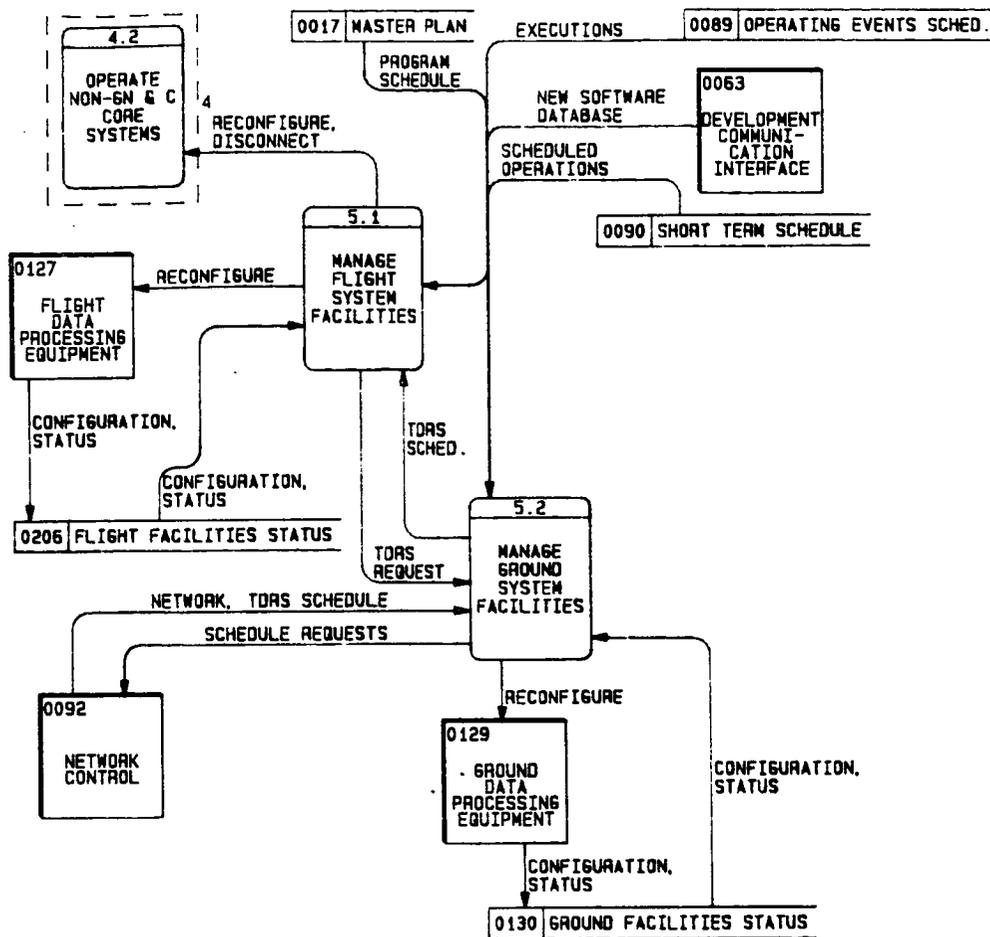
Figure 6-6. SSDS Level 1 DFD 5.0 Manage Facilities and Resources
