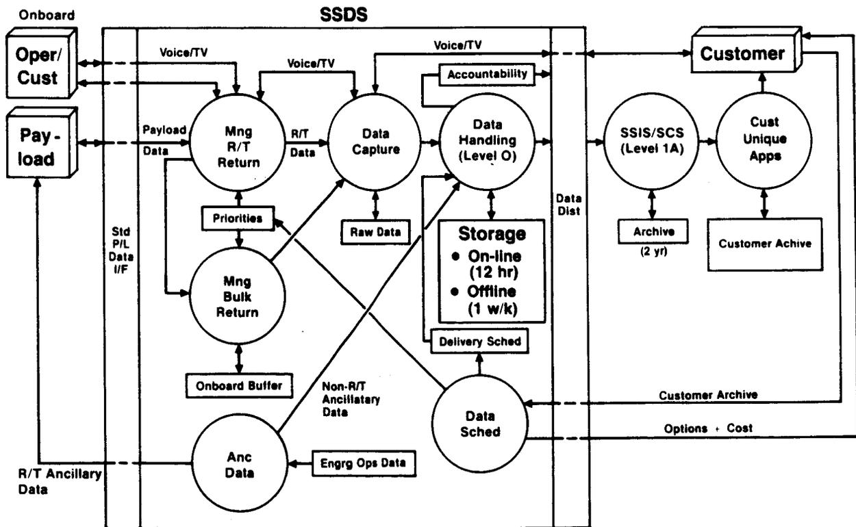
Figure 4-16. End-to-End Customer Data Delivery
