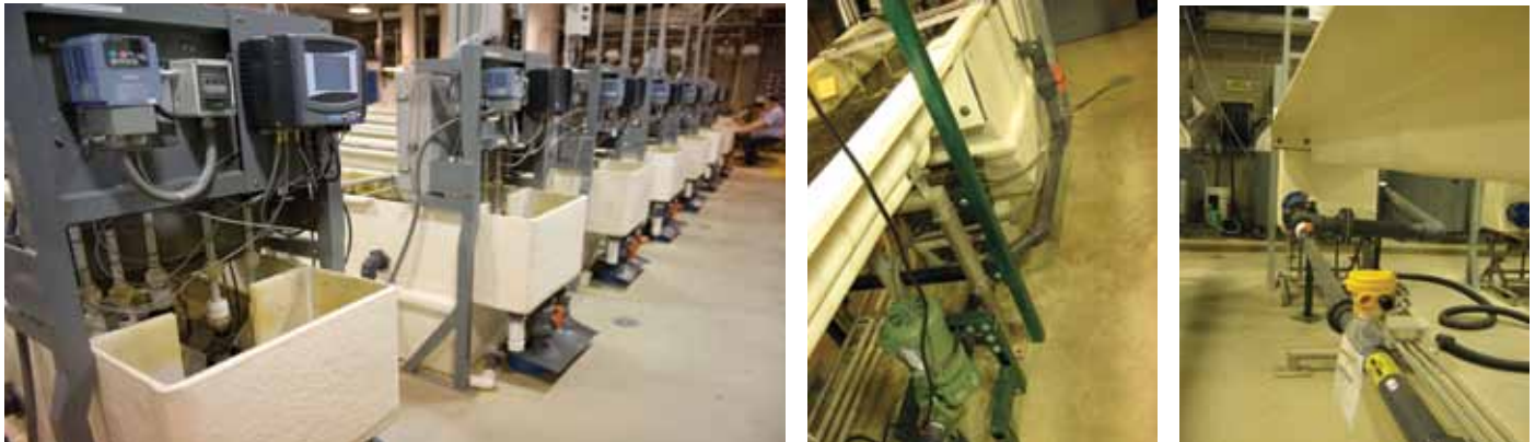
1. Tail tanks 2. Recirculation line from tail tank to pump 3. Flow meter on recirculation loop
