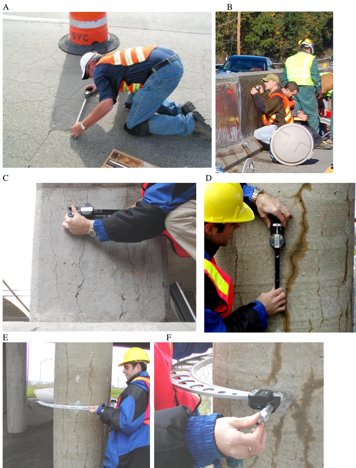
Figure D2. (A). Length-change measurements in a concrete pavement affected by ASR. (B). Length-change measurements in a concrete highway barrier wall affected by ASR. (C to F). Length-change measurements in reinforced concrete columns affected by ASR.
