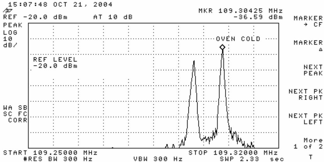
Figure 1 - Test Point 2 LOC Signal
