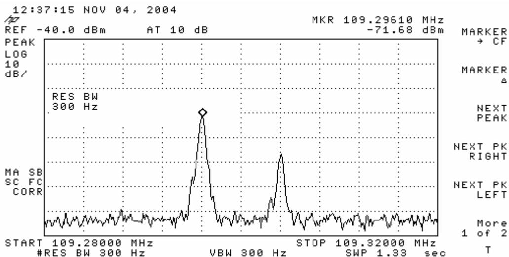
Figure 31 - Test Point 5 LOC Signal
