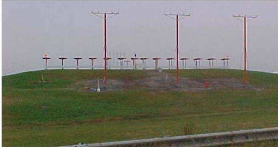
Figure 8 - Localizer Near Atlanta Test Point 2
