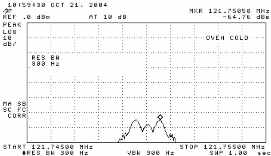
Figure 14 - Test Point 8 VHF Signal
