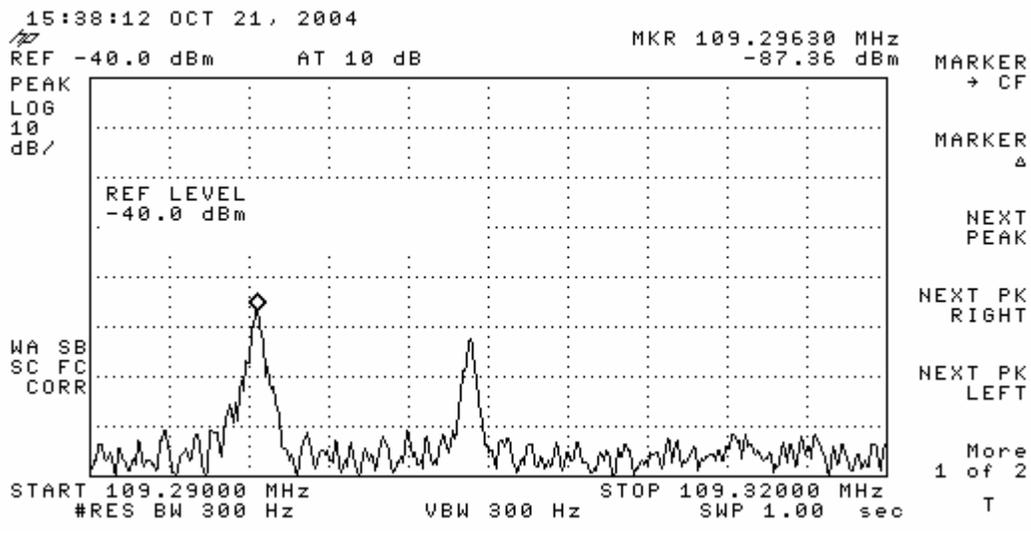
Figure 5 - Test Point 7 LOC Signal
