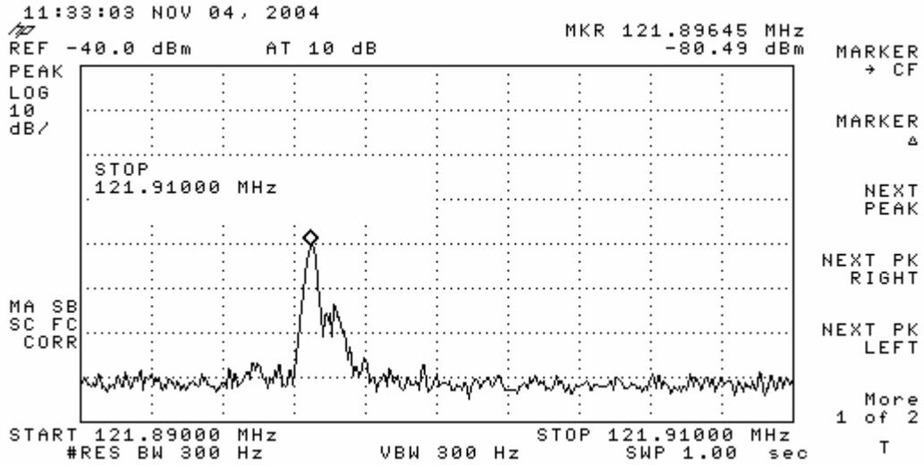
Figure 39 - Test Point 1 VHF Signal
