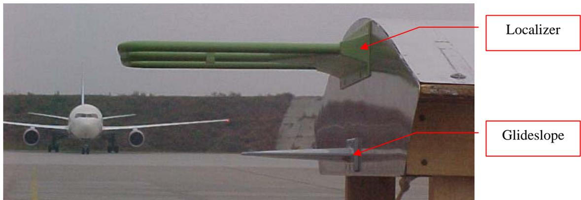
**Figure 3 – Close-up of Antenna Mockup**
