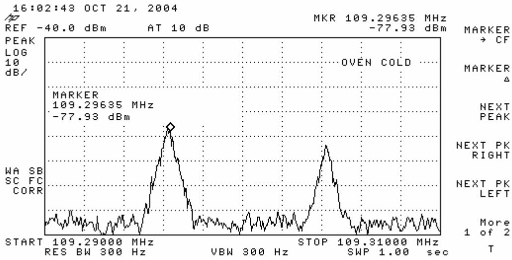
Figure 6 - Test Point 8 LOC Signal
