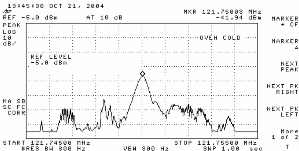
Figure 16 - Test Point 10 VHF Signal
