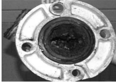
Figure 2: Clogged and Corroded Piping in the NCC
