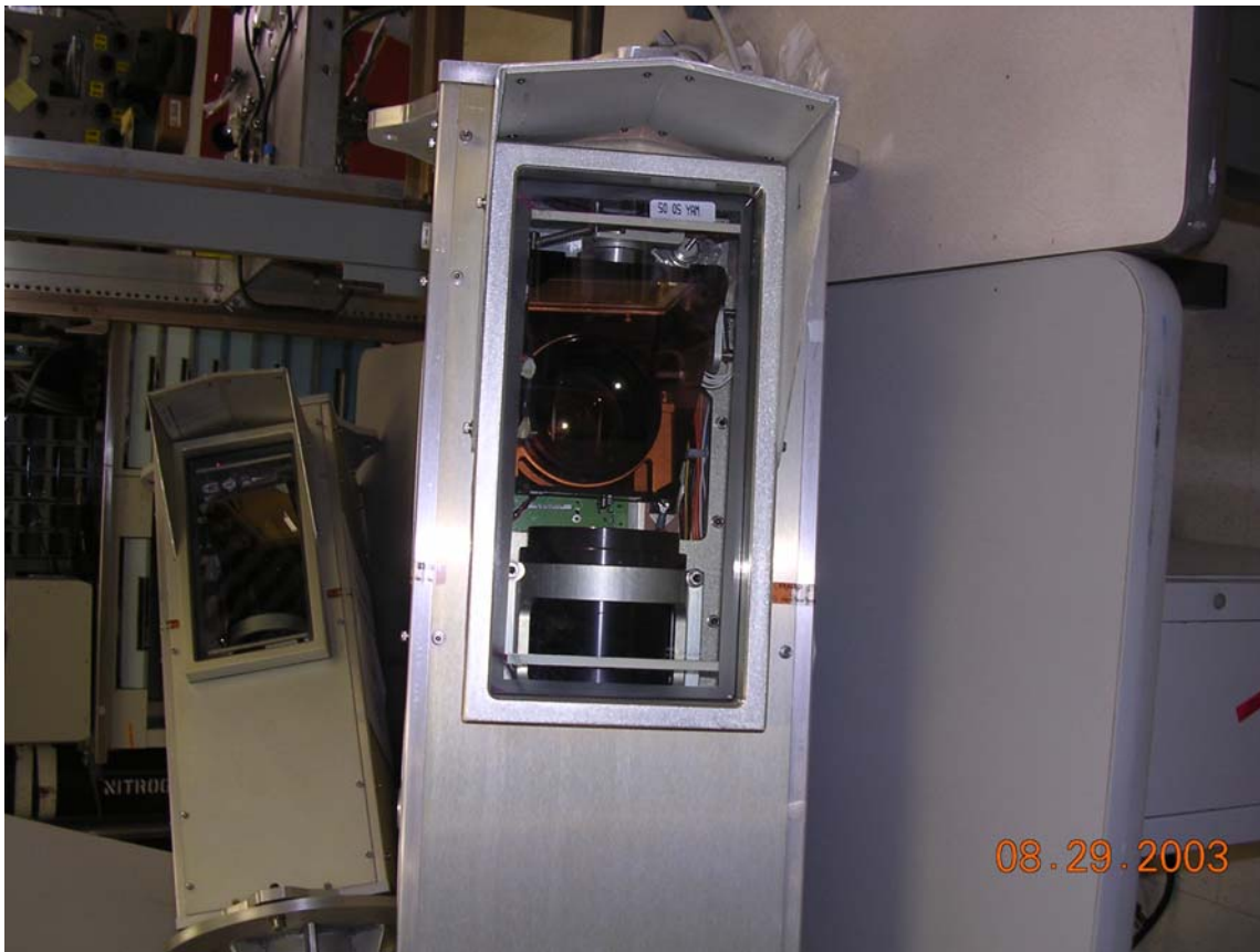
Figure 2-23 AirFiber 5800 With Fiberglass Shroud Removed
