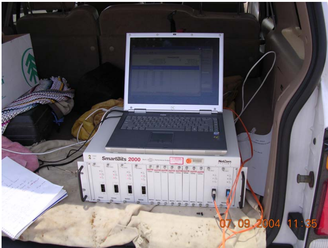
Figure 2-24 Field Testing with the SmartBits & a Laptop
