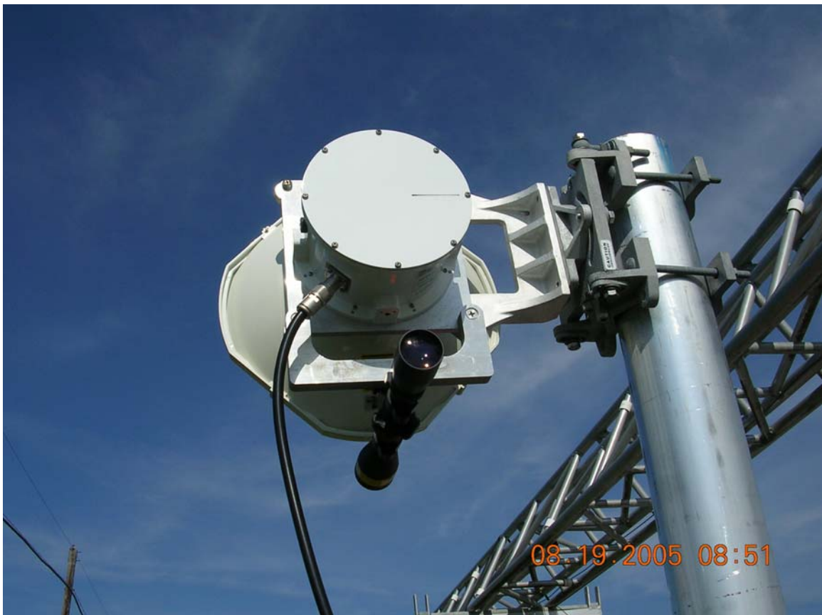
Figure 3-3 Modified AirPair 100 Radio with 30cm Antenna & Added Riflescope
