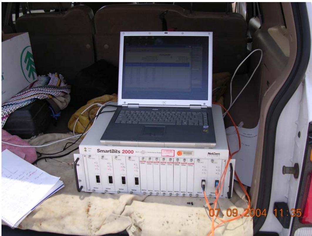
Figure 2-22 Field Testing with the SmartBits & a Laptop
