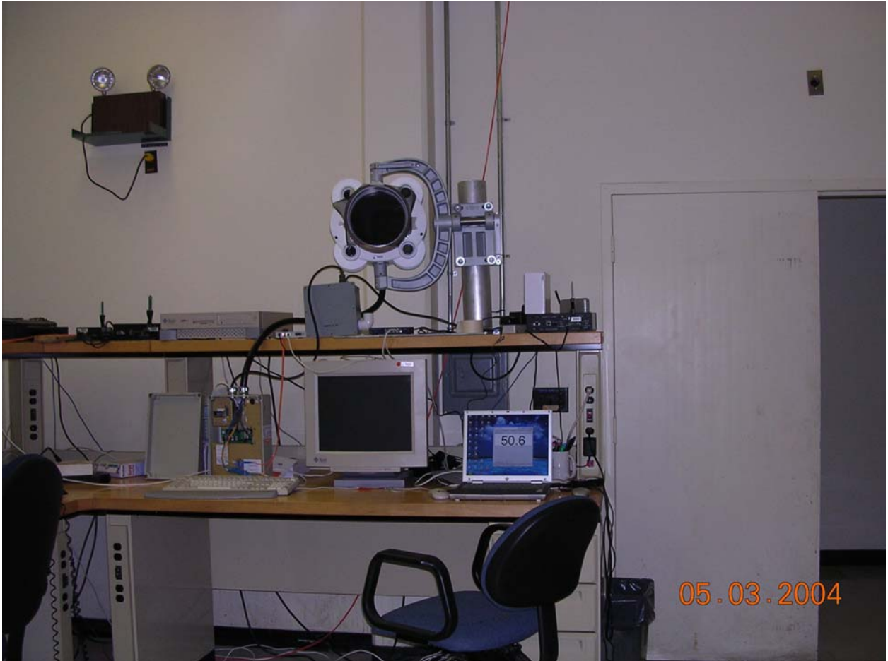
Figure 2-4 OTU #1 with Laptop Measuring Receiver Performance
