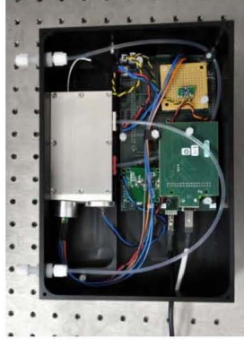
VCSEL-WMS CO detector. 2.3 mm VCSEL absorption-based sensor (0.5 ppm CO)
