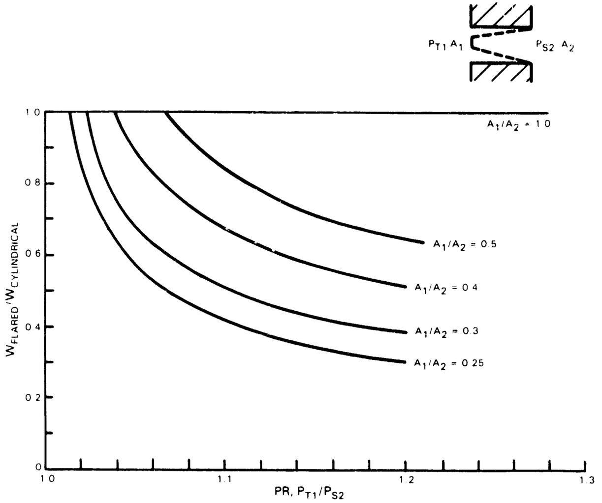
Figure 5-36 Conical Holes Cooling Air Flow Rates
