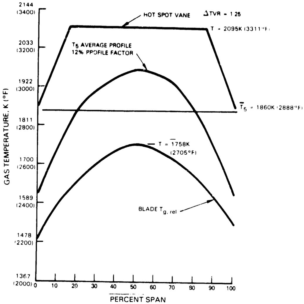
Figure 5-22 Design Gas Temperature Profile = 1986 technology
