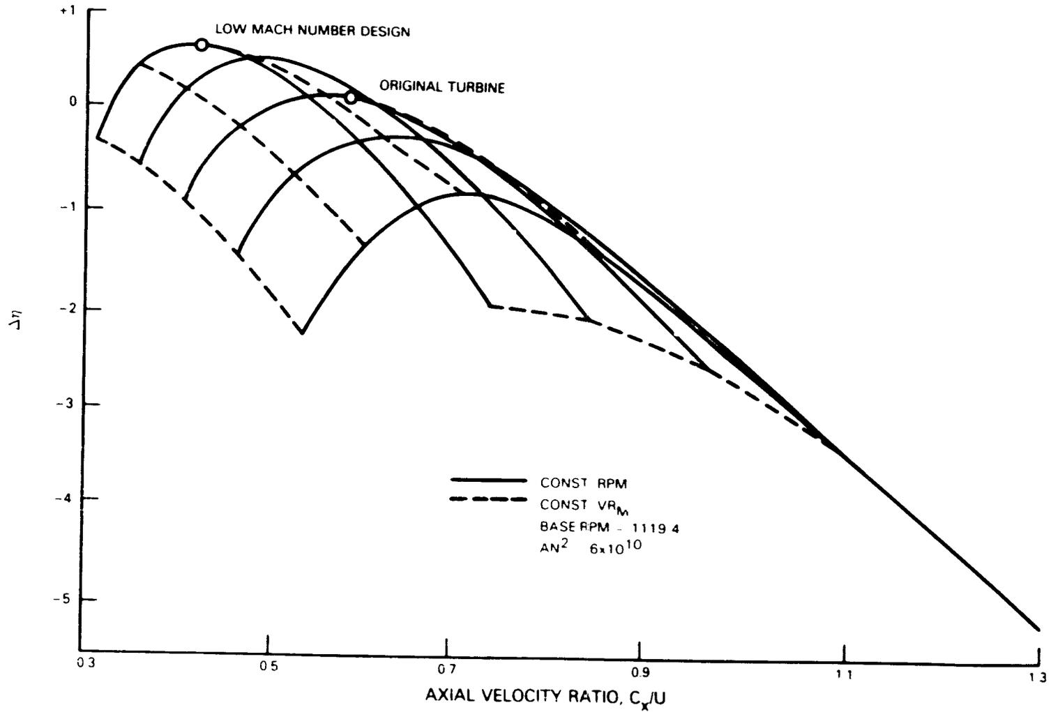
Figure 4-3 High-Pressure Turbine Parametric Study Identified Improved Design
