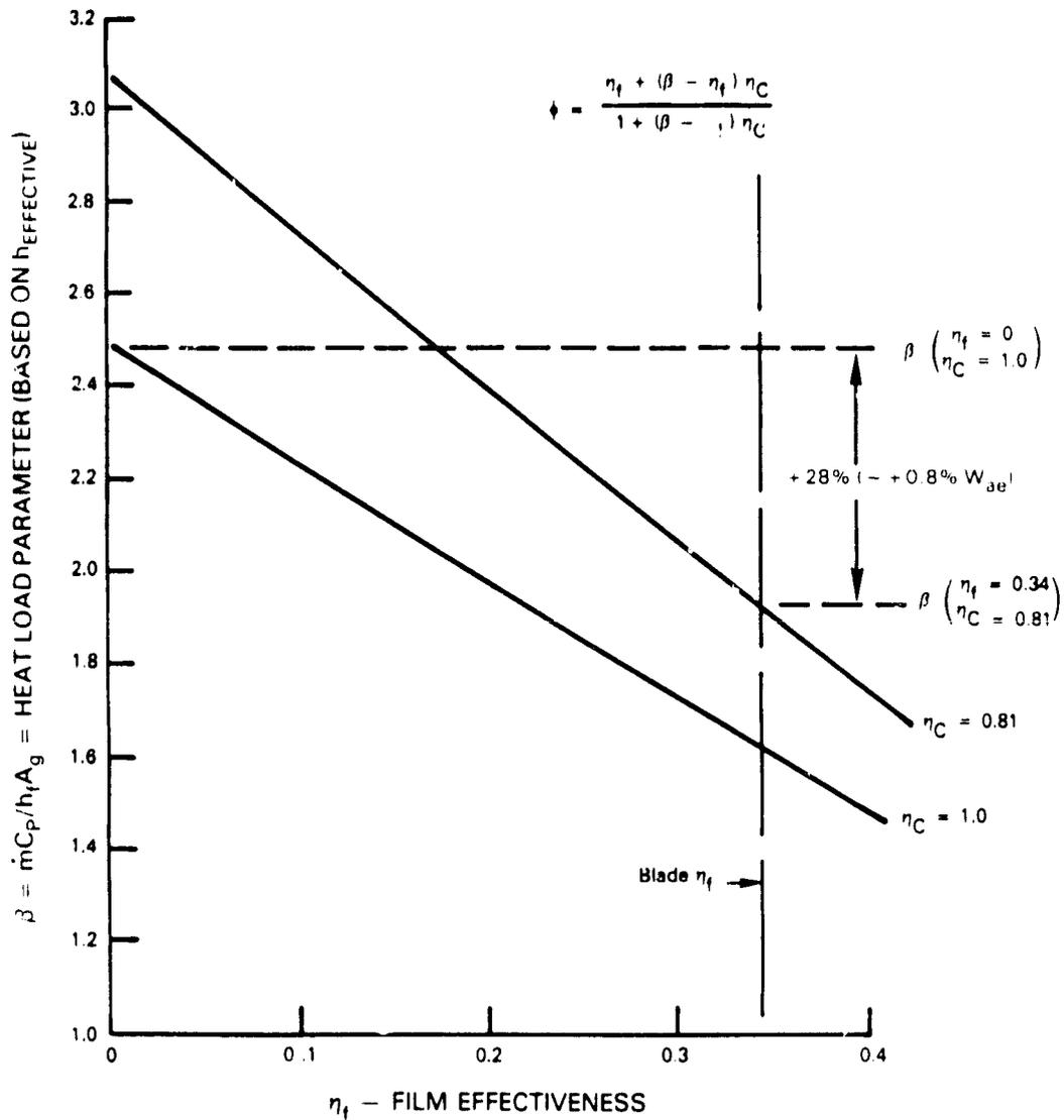
Figure 5-15 Heat Load Parameter vs Film Effectiveness; Blade  $\phi = 0.713$ ,
