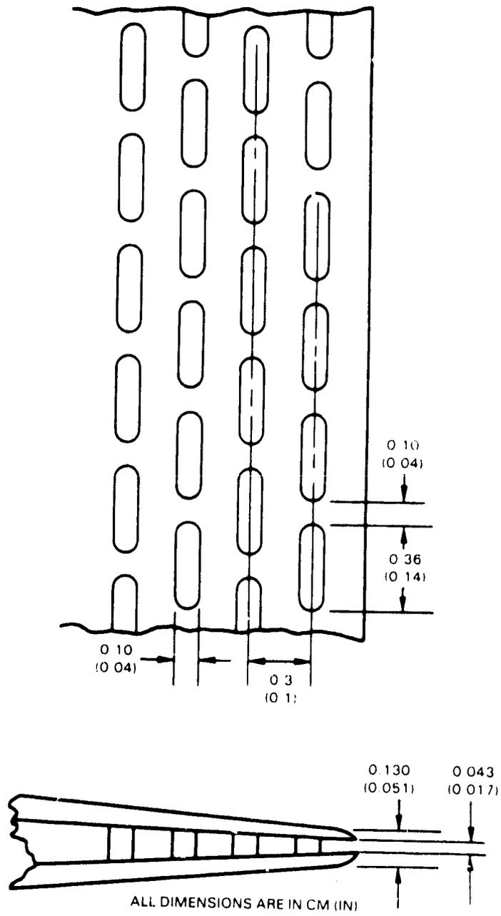
Figure 5-43 Blade Trailing Edge Cooling Configuration (Representative Geometry)
