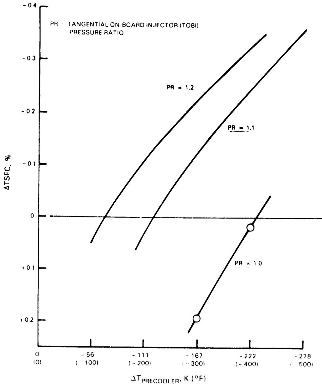
Figure 5-9 Influence on Thrust Specific Fuel Consumption Change of Vane Precooled Airflow from Leading Edge to Blade Cooling With No Weight Penalty
