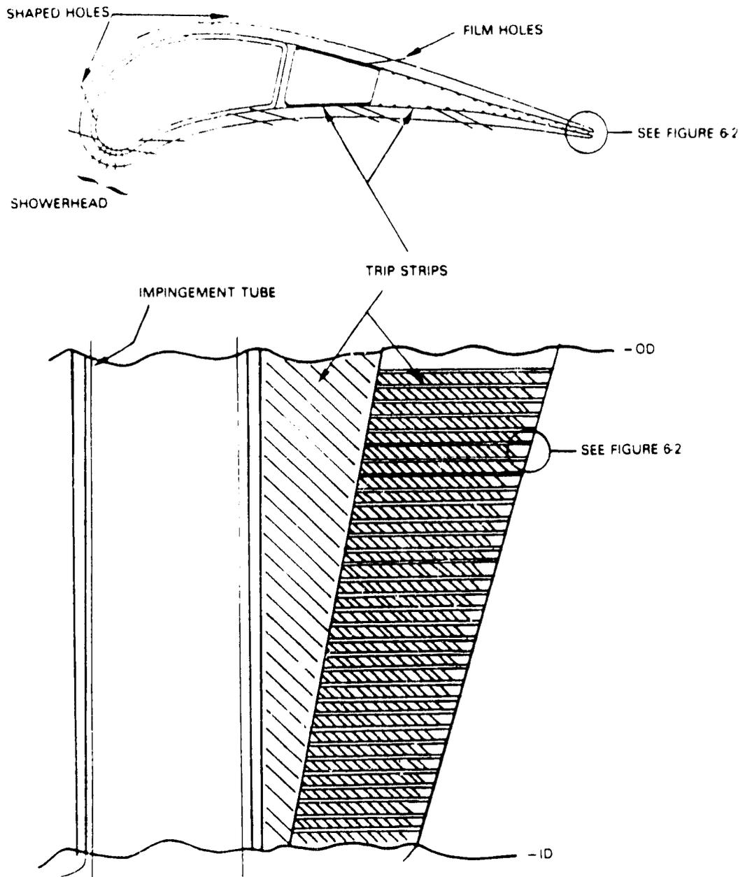
Figure 5-28 vane Cooling Configuration
