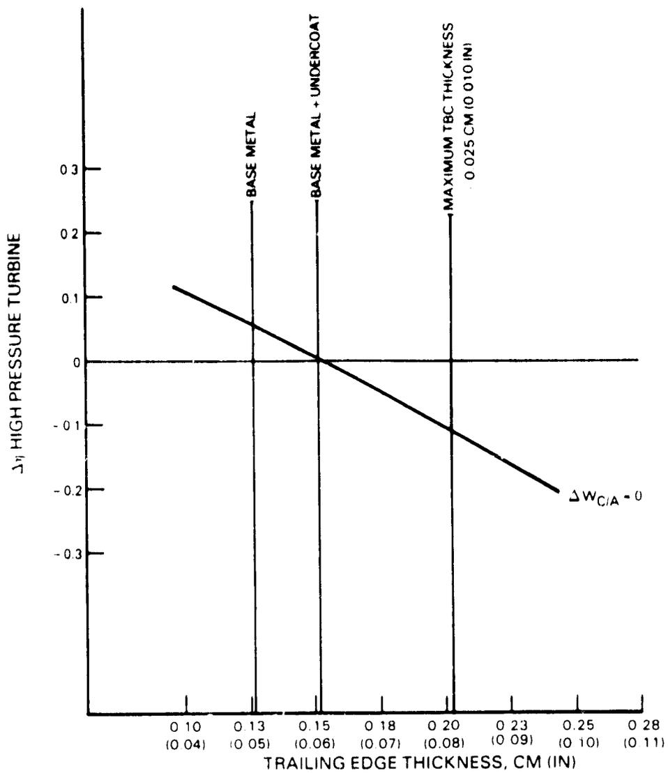
Figure 5-46 First Blade Trailing Edge Thickness Efficiency Sensitivity
