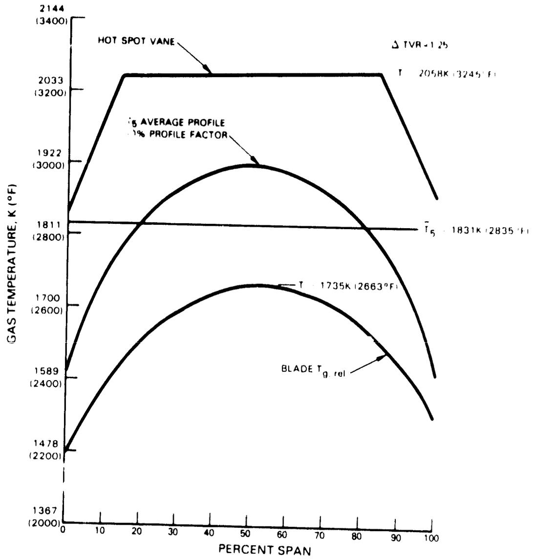
Figure 5-21 Design Gas Temperature Profile = 1990 Technology
