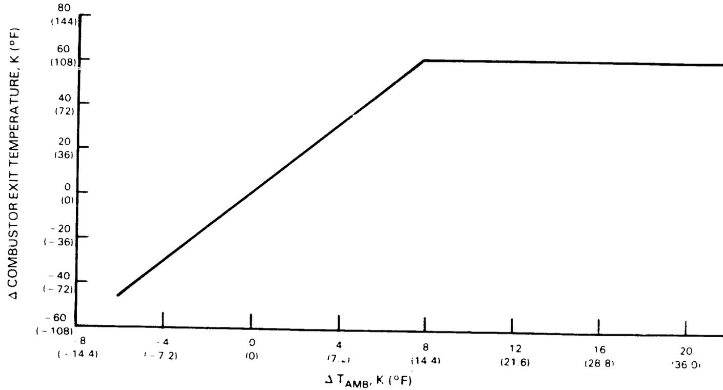
Figure 5-25 Variation of Combustor Exit Temperature as a Function of Variation of the Ambient Temperature
