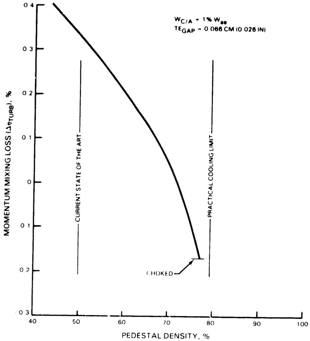
Figure 5-44 Blade Trailing Edge Cooling Losses vs Blockage
