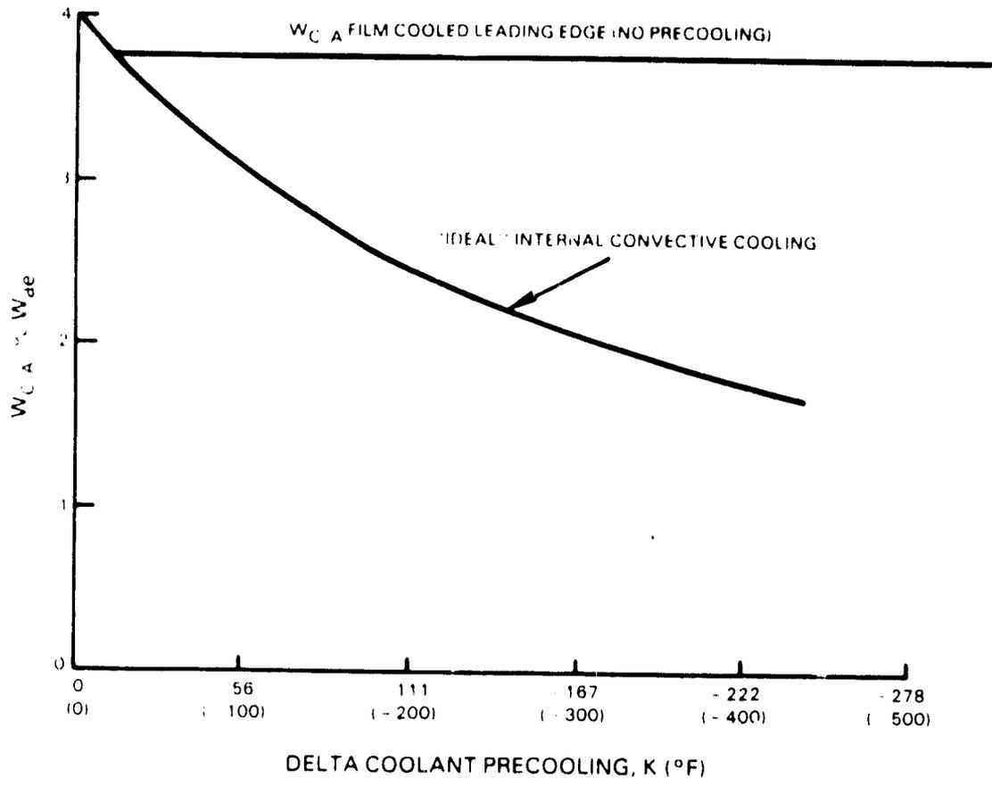
Figure 5-5 Vane Leading Edge Convective Cooling; Effect of Precooling on Coolant Flow
