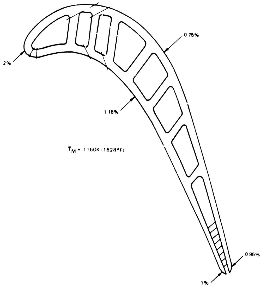
Figure 5-57 Blade Creep at Critical Locations (1986 Technology)
