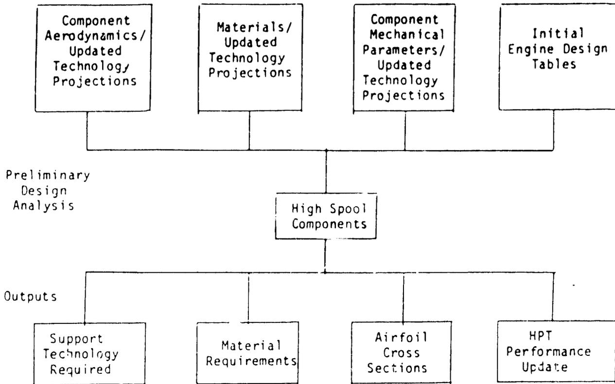
Figure 4-1 Primary Elements of the Preliminary Design Process
