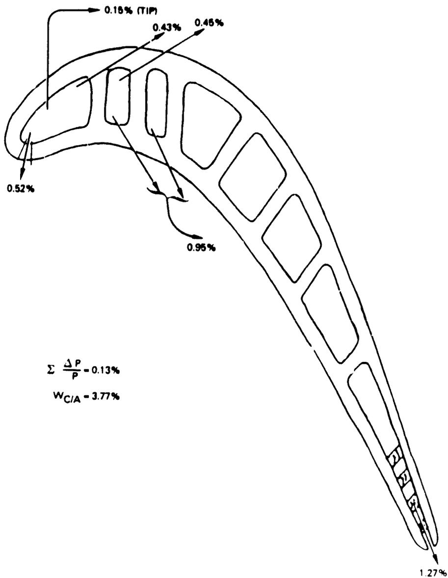
Figure 5-58 Cooling Flow Distribution (1986 Technology)
