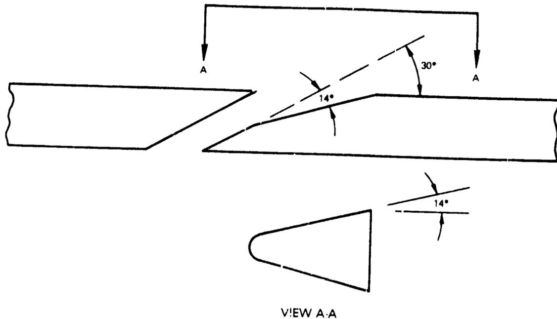
Figure 5-33 Geometry of Suction Surface Shaped Holes
