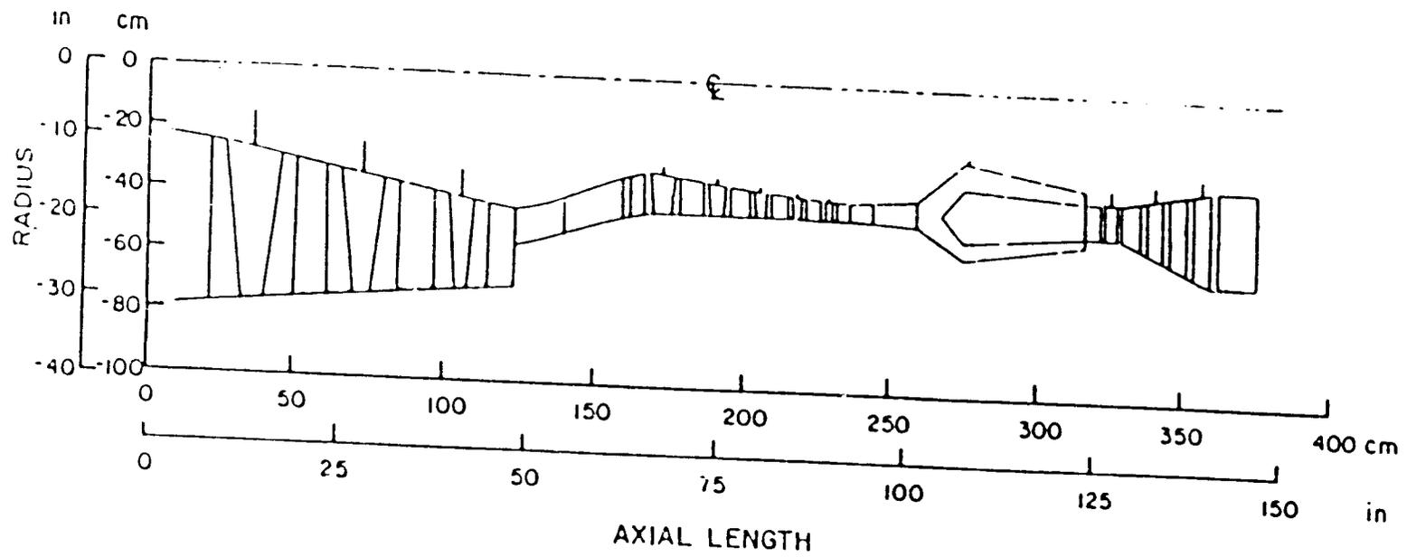
Figure 3-1 Variable Stream Control Engine Flowpath
