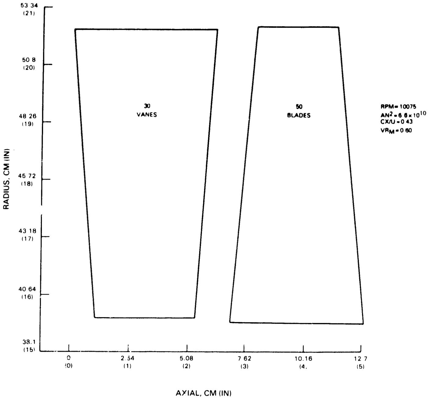
Figure 4-5 Turbine Geometry
