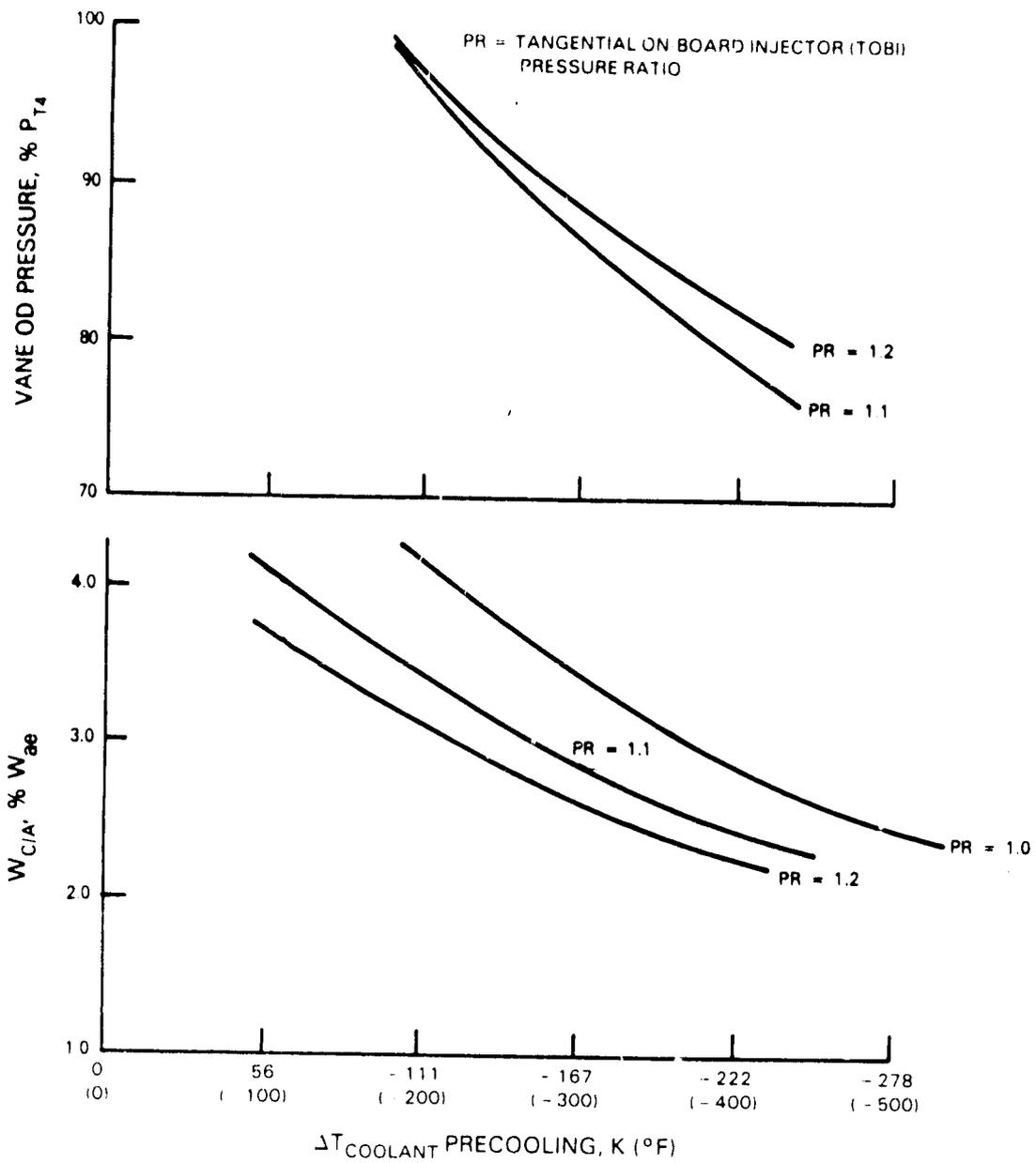
Figure 5-8 Vane Leading Edge Convective Cooling; Coolant Flow vs Precooling
