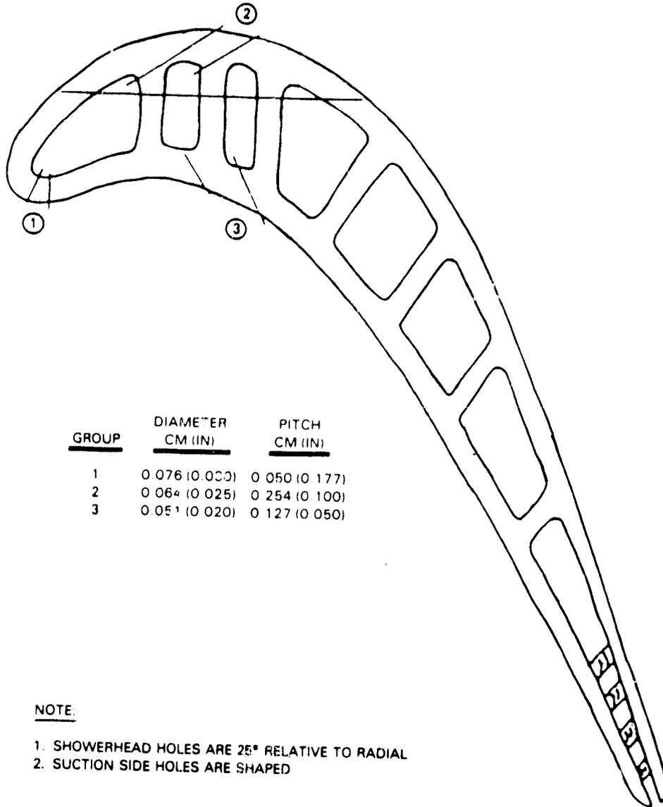
Figure 5-52 Blade Hole Geometry (1990 Technology)
