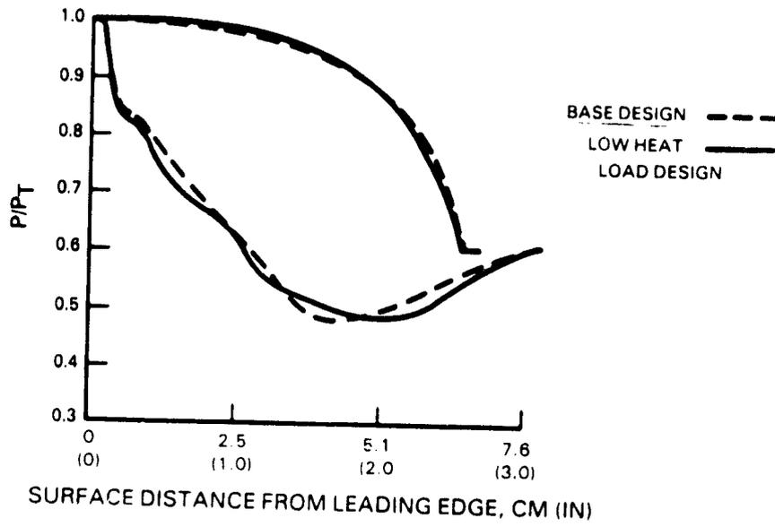
Figure 5-18 Blade Loading for Low Heat Load Design
