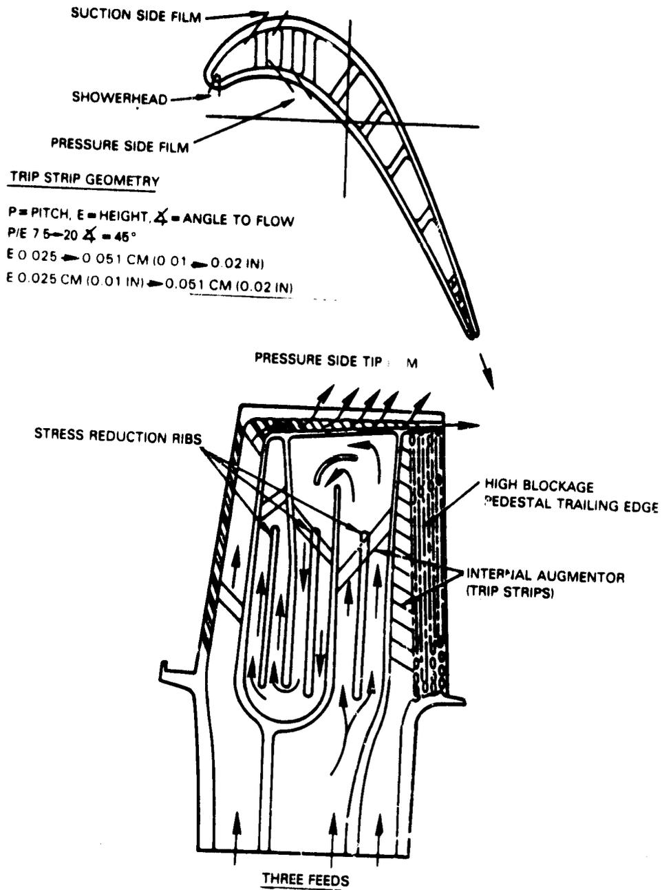
Figure 5-42 Blade Cooling Configuration
