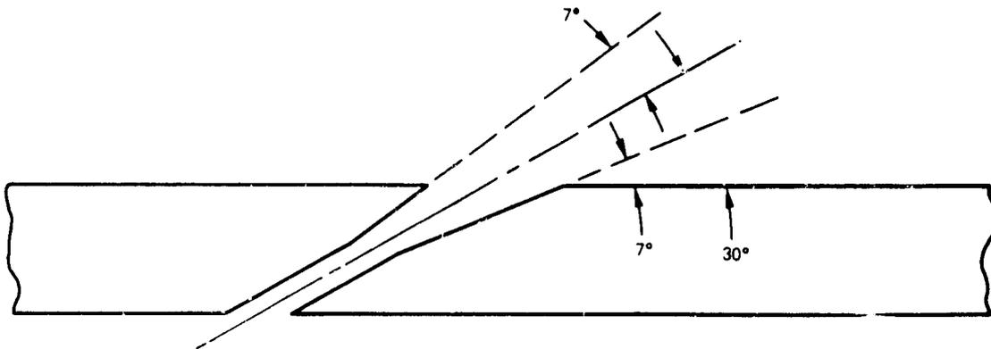
Figure 5-35 Geometry of Conical Showerhead Holes
