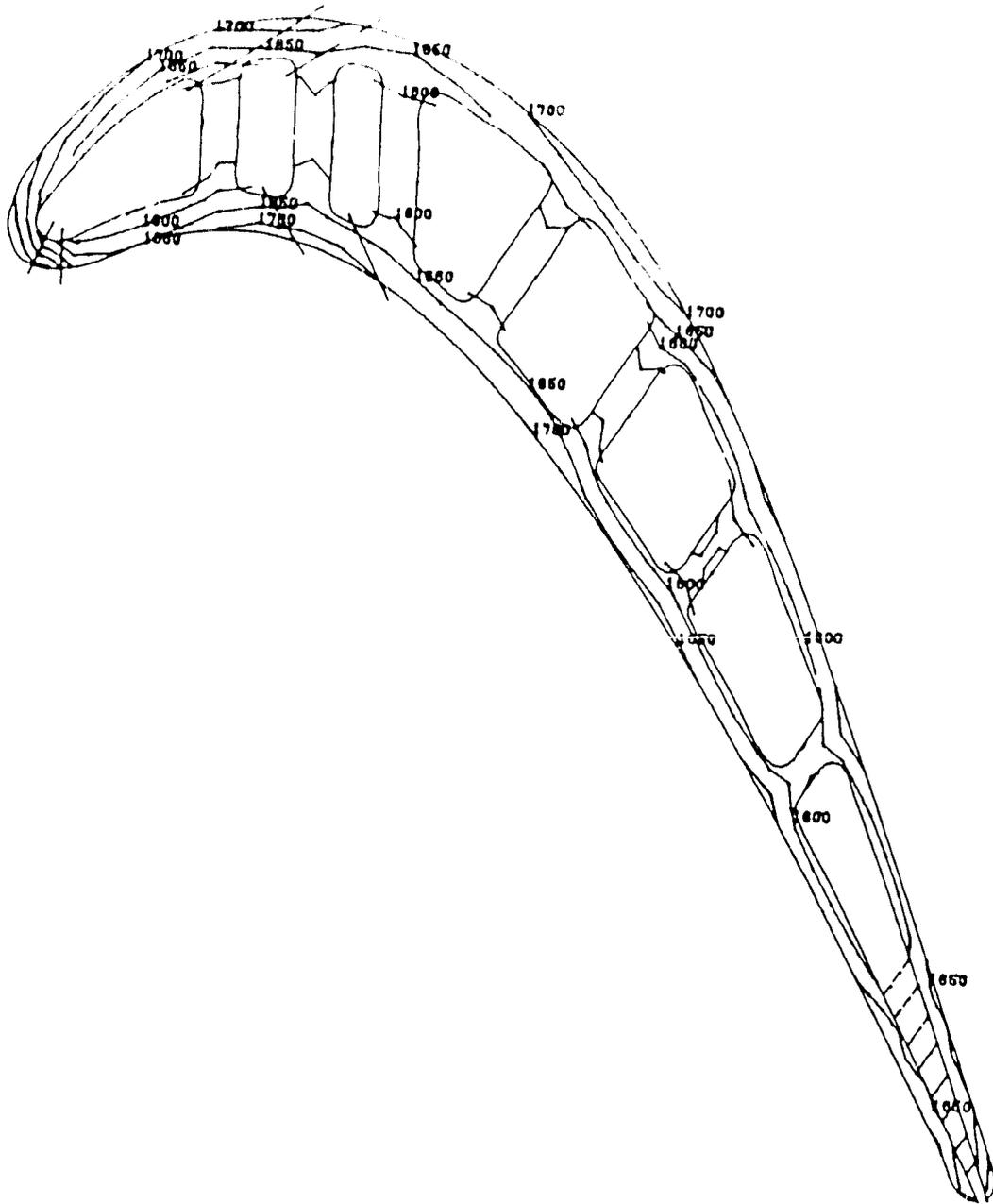
Figure 5-54 Blade Mean Section Isothermals Based on 1986 Technology
