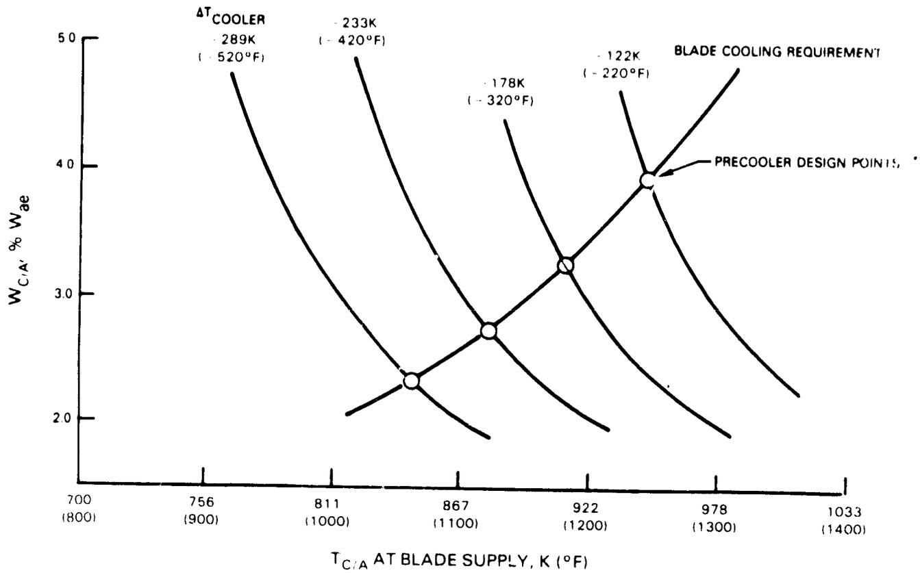
Figure 5-7 Vane Leading Edge Convective Cooling; Coolant Flow vs Temperature
