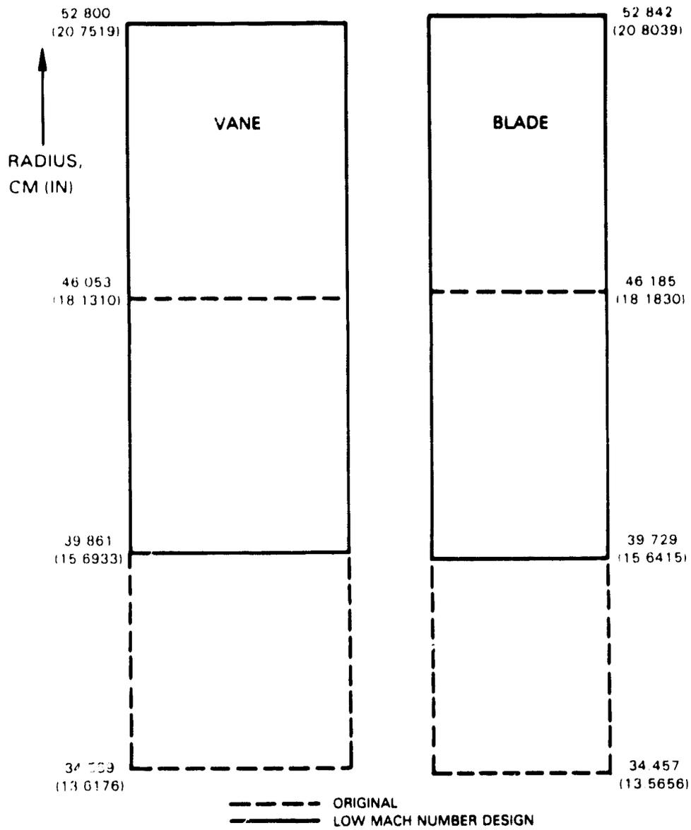
Figure 4-4 Comparison of Original and Final Flowpath
