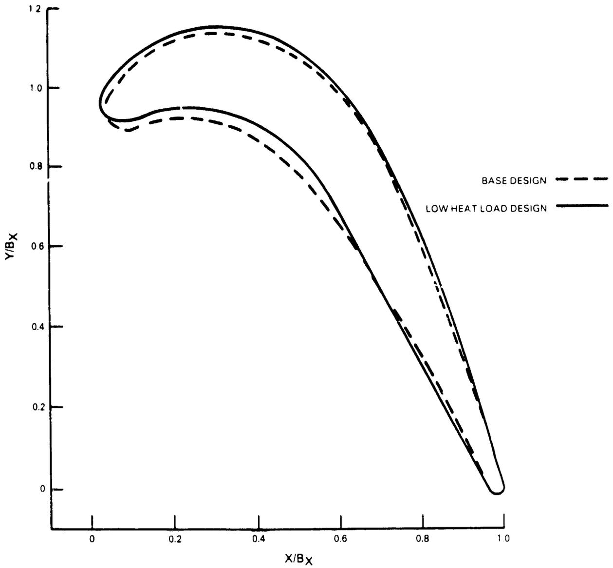
Figure 5-17 Blade Geometry for Low Heat Load Design
