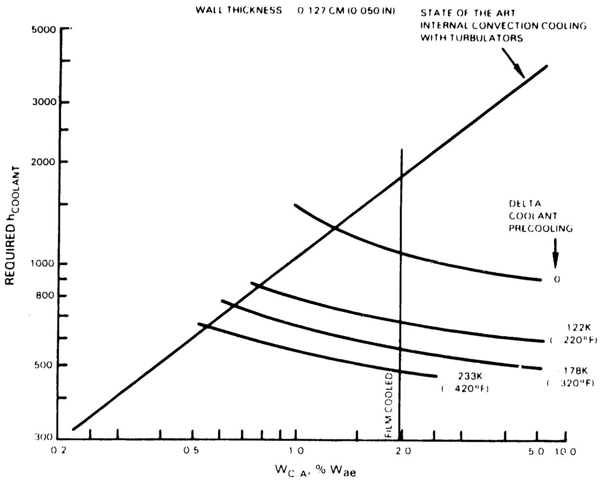
Figure 5-4 Convectively Cooled Vane Leading Edge Using Precooled Air; (Pressure Surface)
