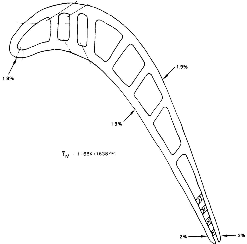
Figure 5-48 Blade Creep at Critical Locations (1990 Technology)
