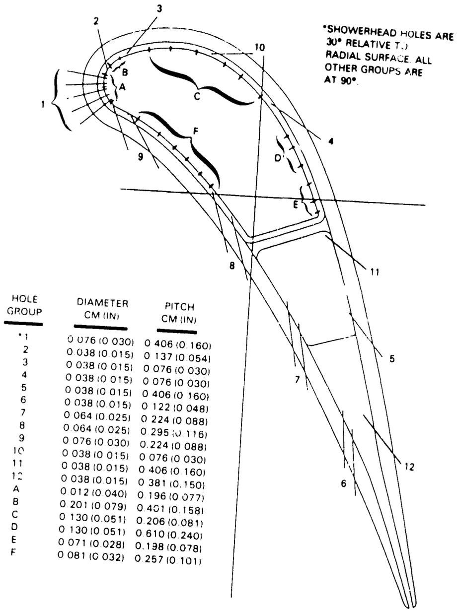
Figure 5-4] Vane Hole Geometry (1986 Technology)
