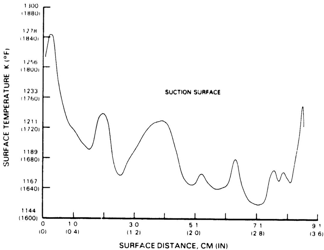
Figure 5-56 Blade Surface Temperature Distribution on Suction Surface (1986 Technology)
