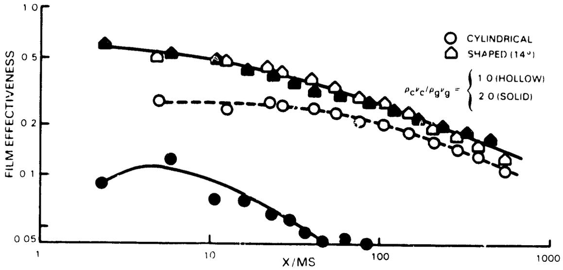
Figure 5-34 Film Effectiveness vs Nondimensional Distance Cylindrical and Shaped Holes
