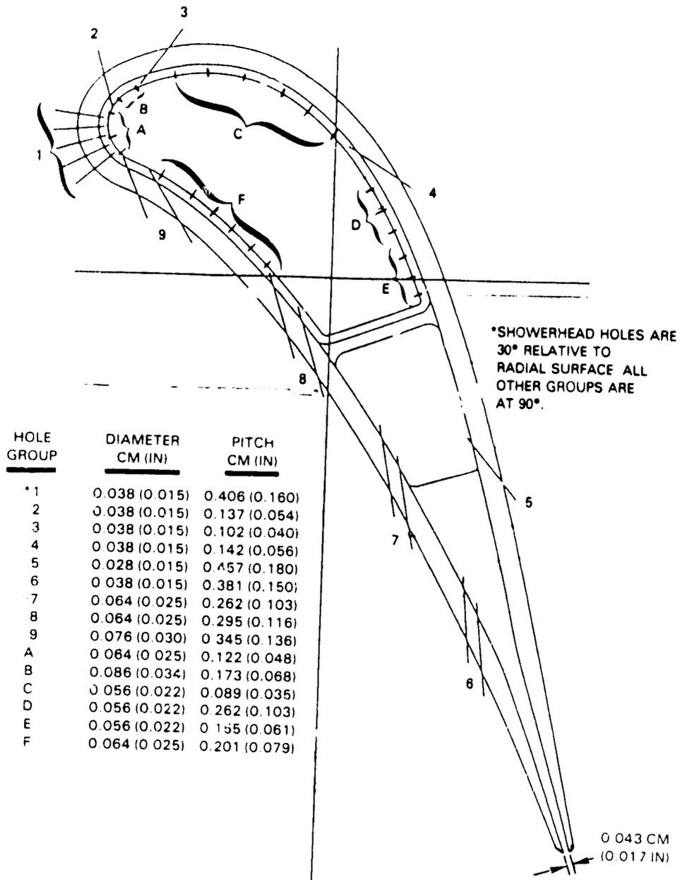
Figure 5-37 Vane Hole Geometry (1990 Technology)
