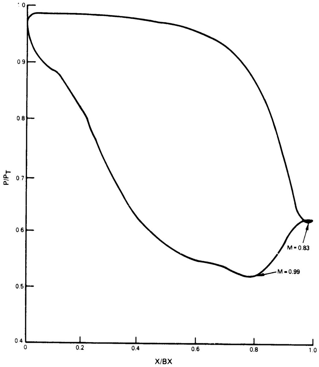
Figure 4-7 Vane (Mean) Pressure Distribution
