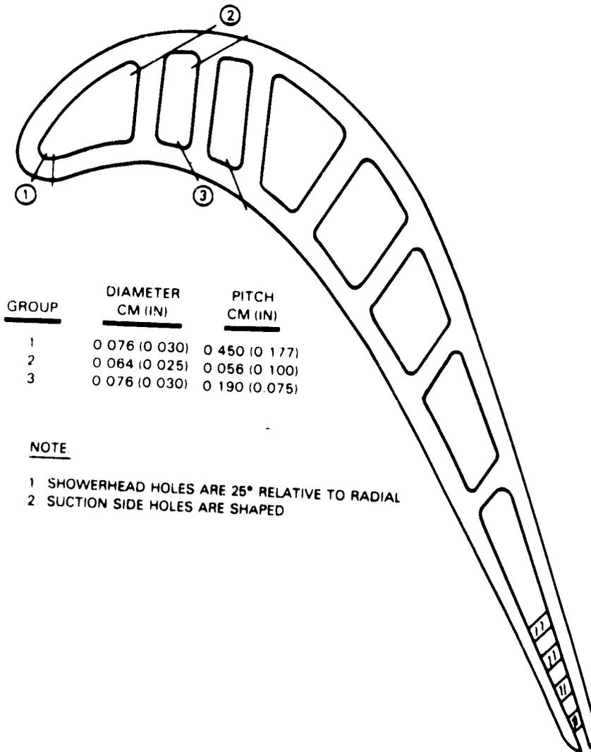
Figure 5-59 Blade Film Hole Geometry (1986 Technology)
