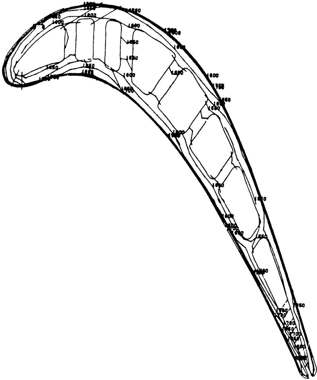
Figure 5-51 Blade Mean Section Isothermals Based on 1990 Technology
