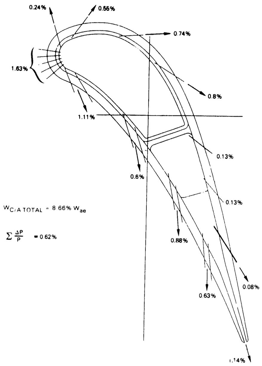
Figure 5-38 Vane Cooling Air Flows (1986 Technology)
