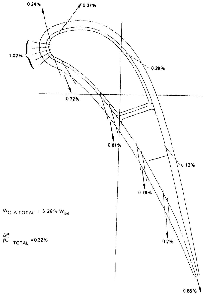
Figure 5-30 Vane Cooling Air Flows (1990 Technology)
