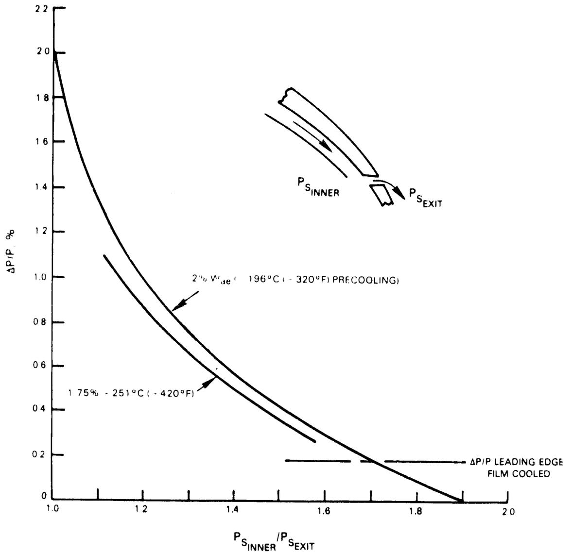
Figure 5-6 Vane Convective Leading Edge; Momentum Mixing vs Exit Pressure Ratio
