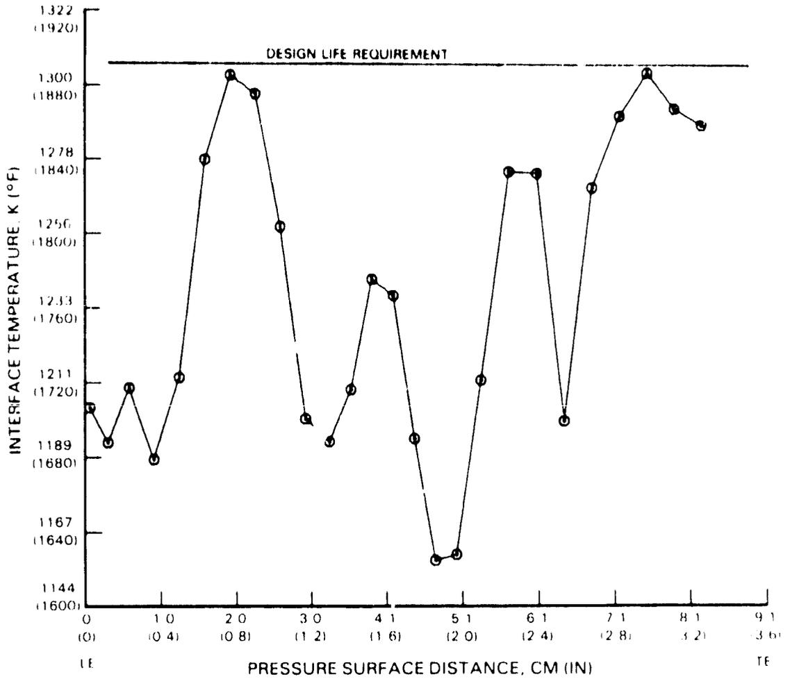
Figure 5-31 Vane Interface Temperature Distribution on Pressure Surface (1990 Technology)
