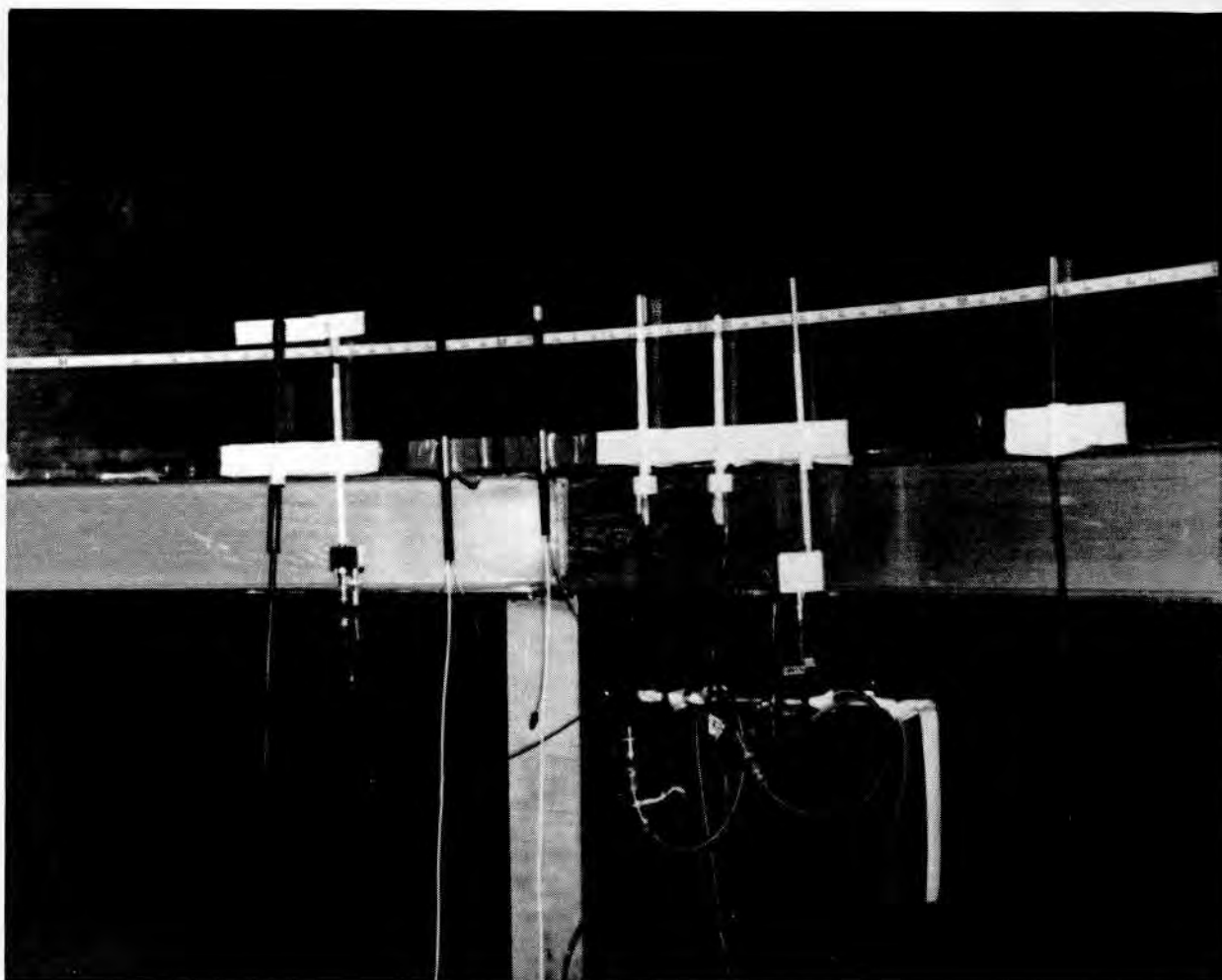
Figure 3. Ionization chambers mounted on the aluminum screen for measurements in free air.
