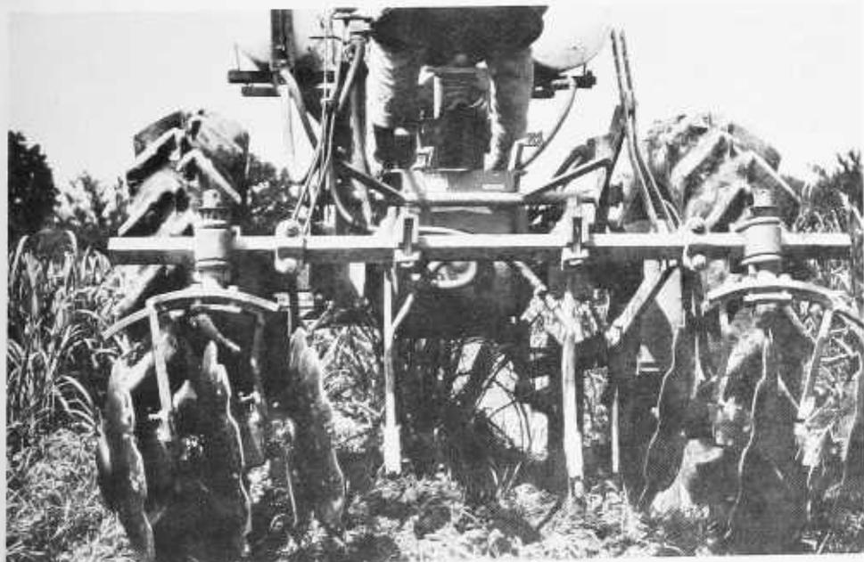
FIGURE 21.—Applying nitrogen in the form of anhydrous ammonia to sugarcane.
