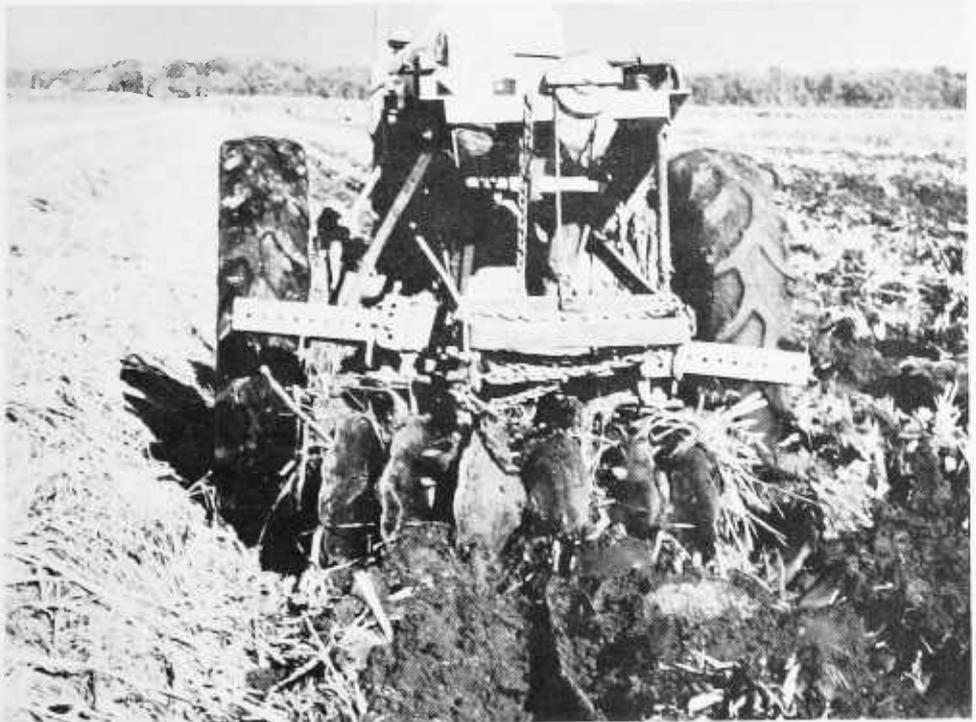
FIGURE 15.—First step in preparing seedbed is destroying old sugarcane stubble.
