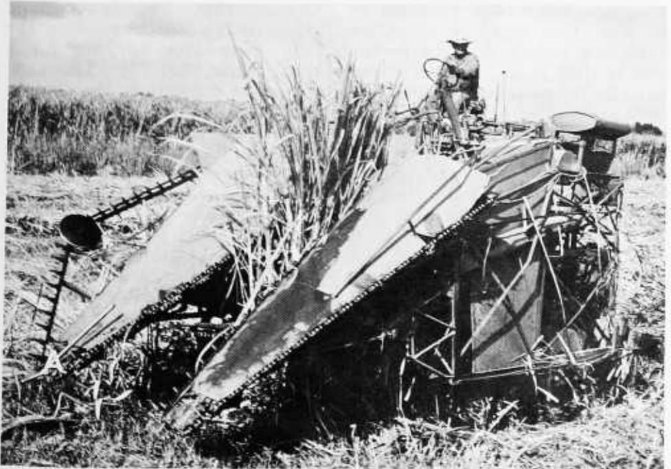
FIGURE 28.—Sugarcane harvester, illustrating pickup attachment (A) for harvesting lodged sugarcane.
