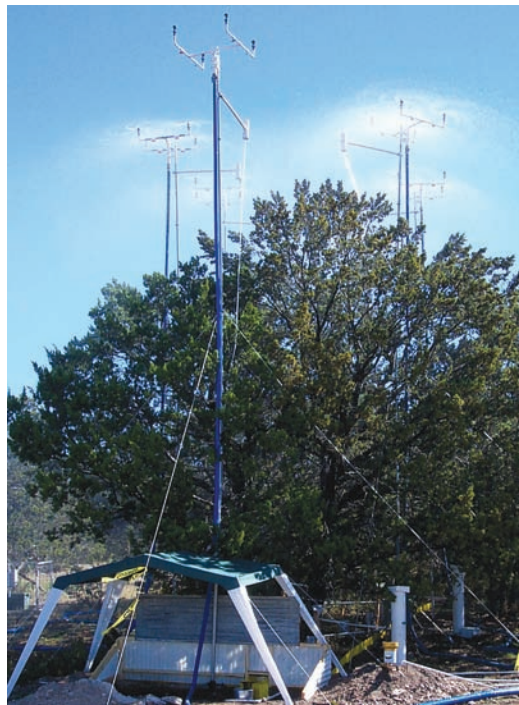
FIGURE 16. Rainfall simulation is a valuable tool for understanding how woody plants alter hydrological properties on rangelands. Large-scale rainfall simulation experiments, like the one conducted here on Ashe juniper rangelands, have the advantage of being able to apply known amounts of water above the tree canopies and enable quantification of canopy interception and water and erosion dynamics at the hillslope scale. (Photo: Bradford Wilcox)
