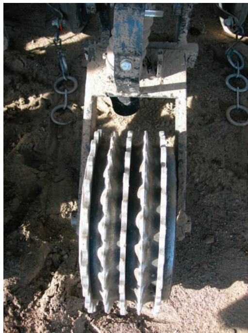
Brillion wheel for pressing broadcast seeds into the soil (Photo: USFS, 2006)
