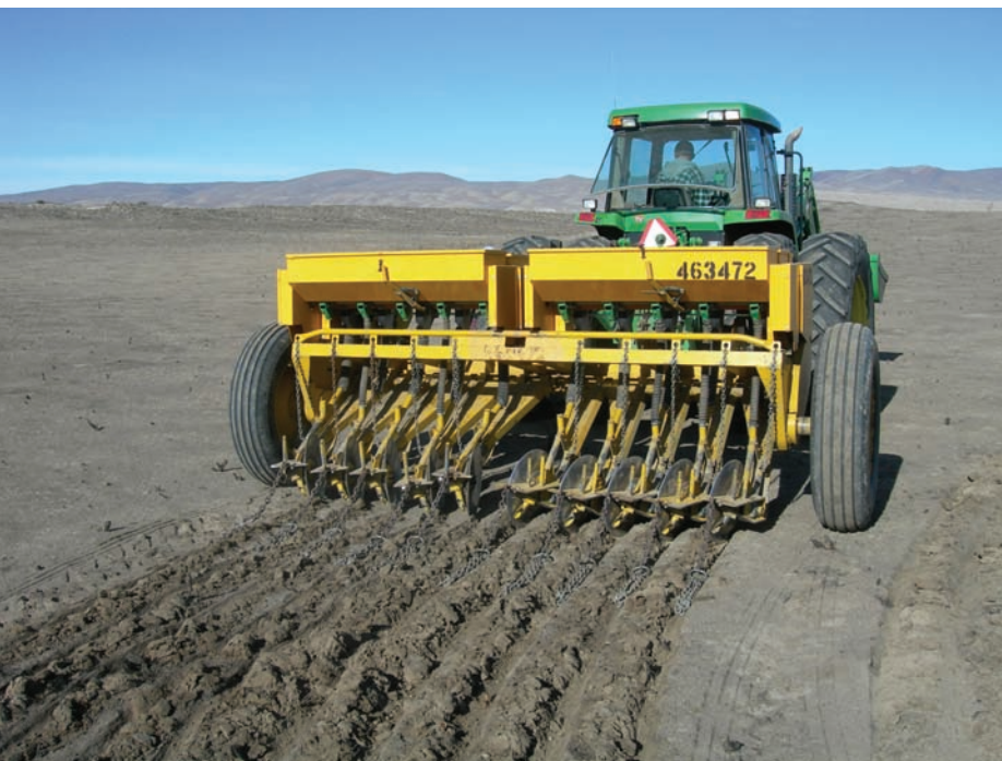
Standard rangeland drill conducting a native seeding following the East Humboldt fire, Elko Co., NV. (Photo: USFS, 2008)
