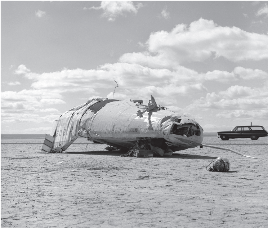
The wreckage of the M2-F2 lies on its back on Rogers Dry Lake. Bruce Peterson's helmet is visible in the foreground. (NASA)
