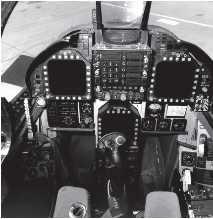
Modern “glass cockpits,” such as in the F-18 Hornet, feature electronic multifunction displays, which a pilot can adjust and optimize according to need. (NASA)
