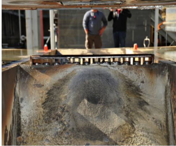
Figure 14. ASMAT below-deck IOP SS (main flame deflector with crest water).
