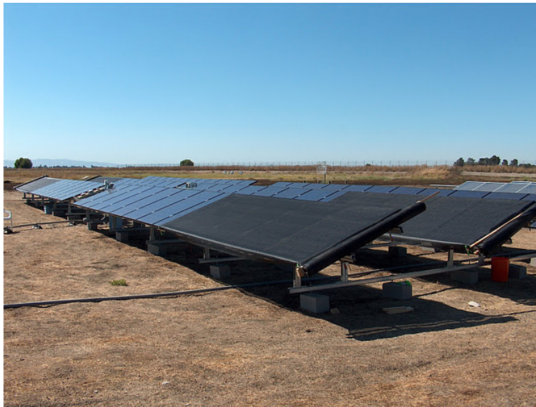
Figure 12. Image showing the two arrays at the test yard in Davis, California. The reference array is on the right, and the Enphase array is on the left. Both arrays are shaded in the (14:14:0) configuration. The irradiance sensors and met station are centrally located in the front row between the two arrays.
