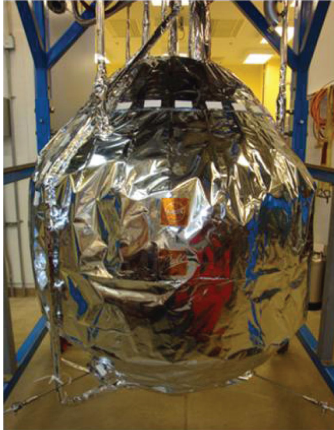
Figure 2.—MLSTC tank insulated with 61 layers of MLI.
