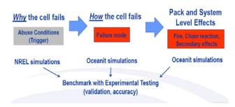
unintended short circuit, the pressure changes are drastic – and often lead to uncontrolled failure of the cells. As part of work for others with Oceanit Laboratories Inc. for the NAVY STTR, NREL built Computational Fluid Dynamic (CFD) simulations that can identify potential weak spots in the battery during such events, as well as propose designs to control violent failure of batteries.
