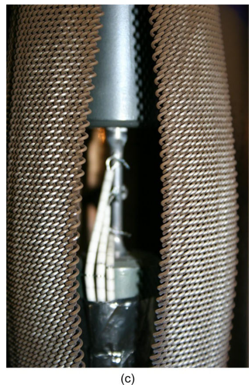
Figure 5.—Brew constant-load creep-test frame. (a) View of frame and chamber. (b) View inside chamber. (c) Thermocouples attached to specimen.
