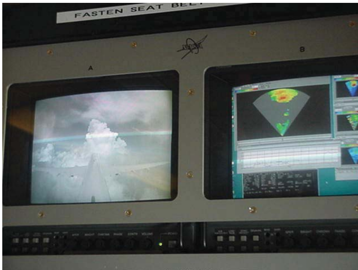
Figure 118. Real-time displays inside ARIES while approaching a turbulence encounter during Flight 235. Video from tail camera displayed on left, and airborne Doppler radar products on right.
