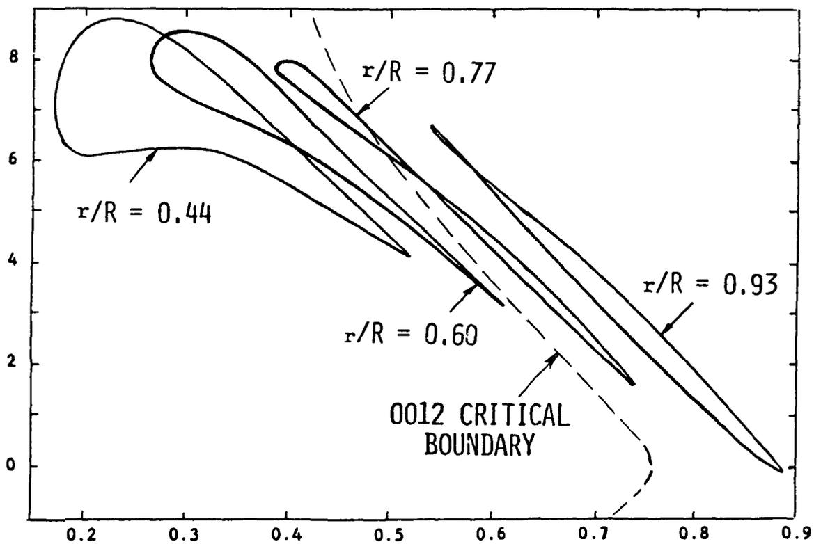
FIGURE 6. TYPICAL RANGES OF CONDITIONS EXPERIENCED BY FOUR SELECTED BLADE STATIONS FOR THE LEVEL FLIGHT CASES.
