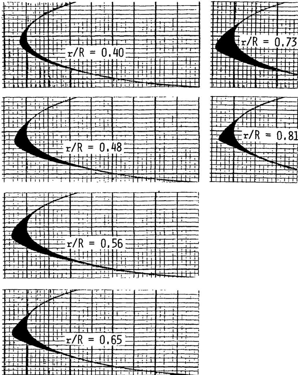
FIGURE 3. PROJECTIONS OF MOLDS OF ICE ACCRETIONS IN LEVEL FLIGHT ( FLIGHT G )
