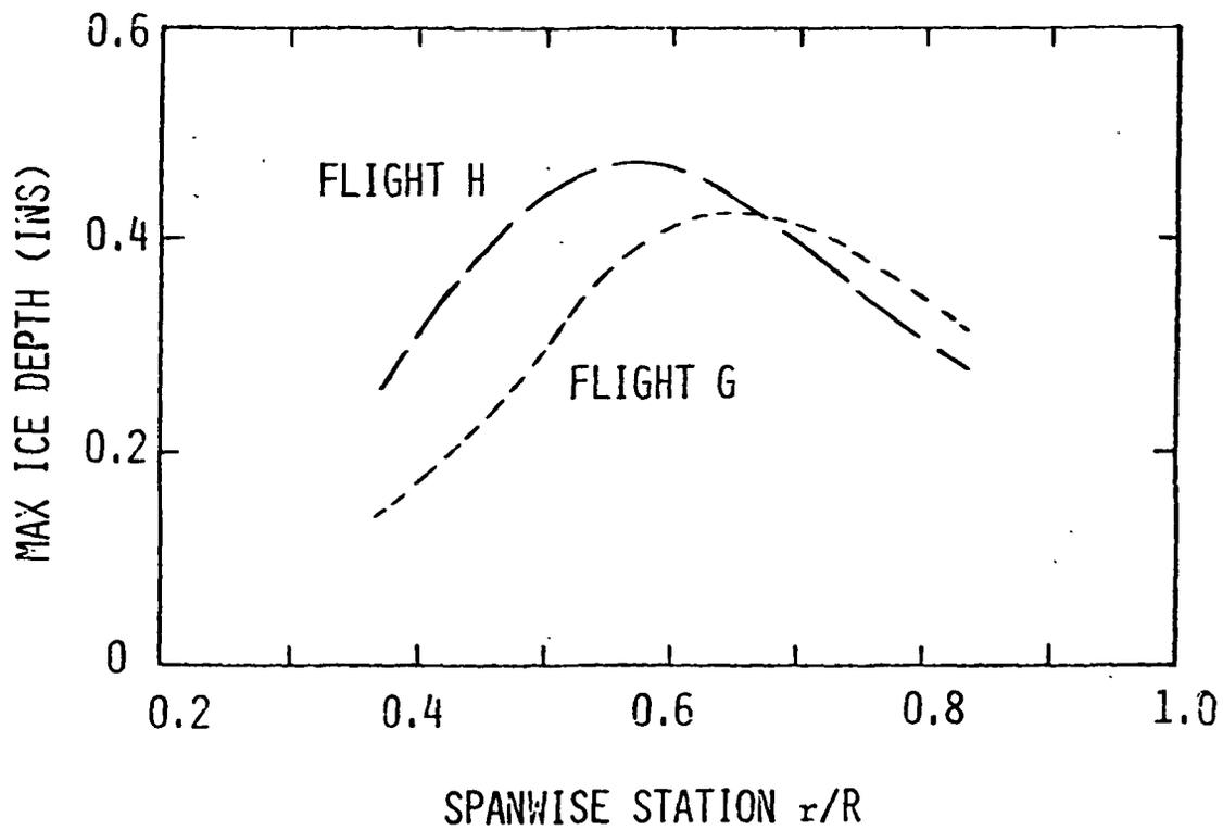
FIGURE 5. DEPTH OF ICE ACCRETED IN LEVEL FLIGHT
