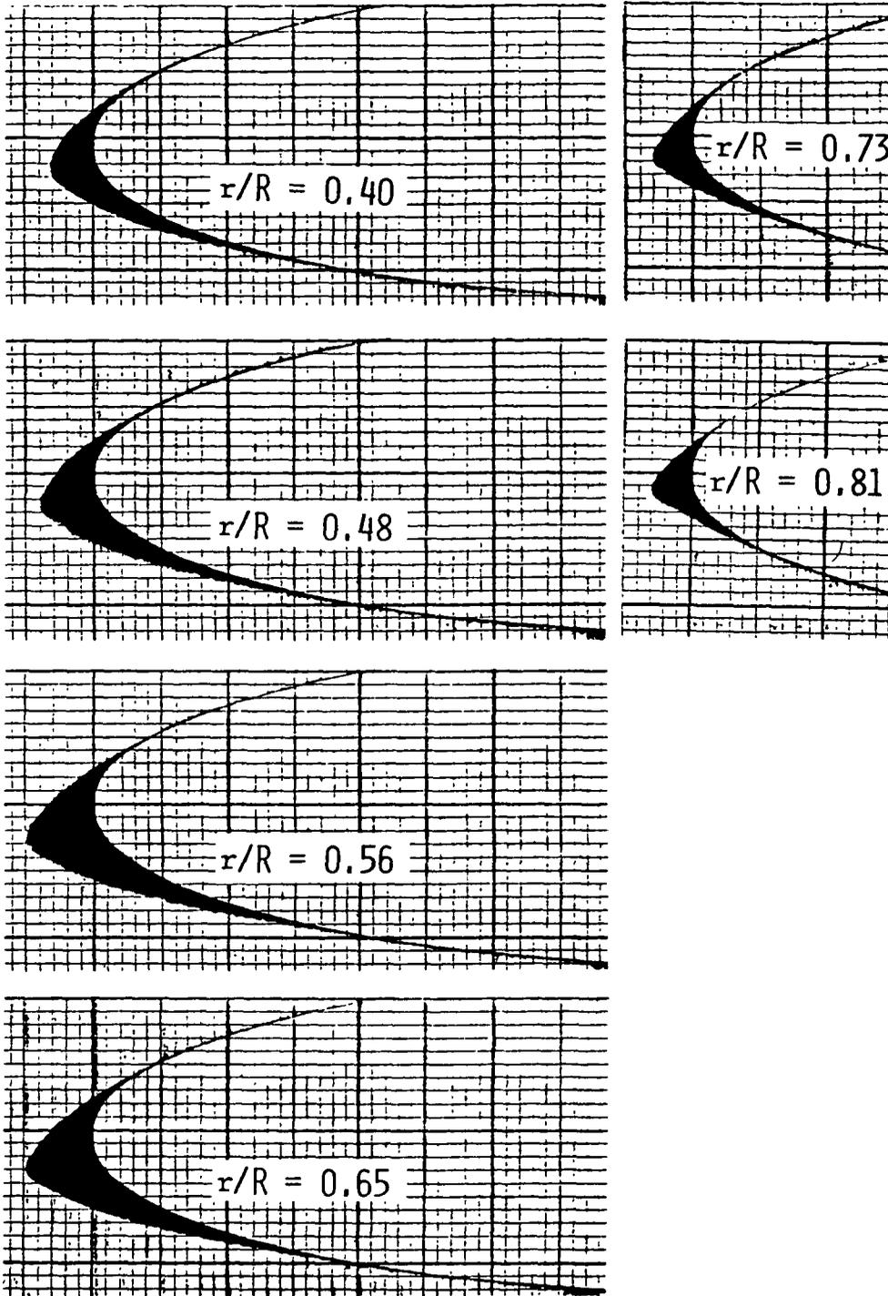
FIGURE 4. PROJECTIONS OF MOLDS OF ICE ACCRETIONS IN LEVEL FLIGHT ( FLIGHT H )
