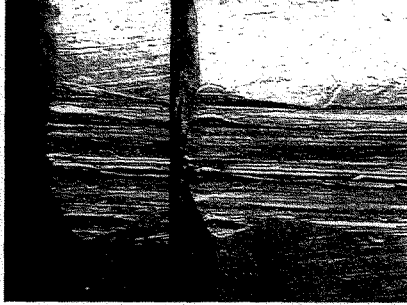
Figure 1 – Comparison of standards from L24184 out of phase by two land impressions.
