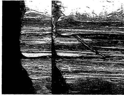
Figure 2 – Comparison of gross marks between barrels L24184 and L24185.
