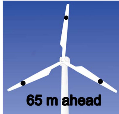
Figure 5. LIDAR configuration A continuous-wave LIDAR scanning pattern provides a preview (65 meters ahead of the turbine) LIDAR measurement of the horizontal wind speed at 75% span for each blade
