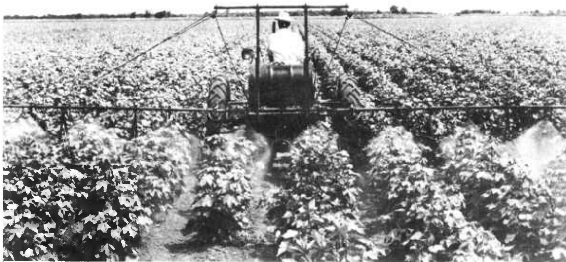
Figure 17.—Eight-row, low-volume, low-pressure spraying machine in operation.
