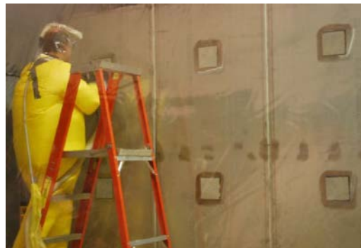
Figure 3-2. Containment tent: outer view (left) and inner view with test stand containing contaminated coupons (right).
