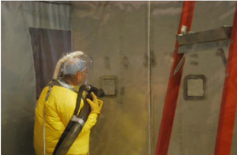
Figure 3-3. Operator applying Blast N'Vac to concrete coupon.
