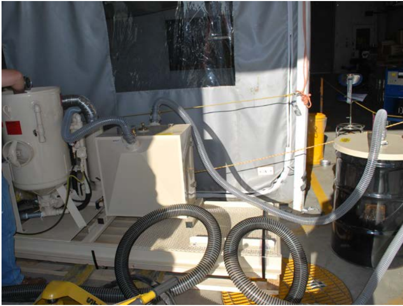
Figure 2-2. Blast N'Vac abrasive grit reservoir, HEPA filter, and collection drum.
