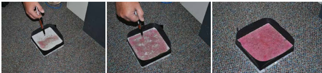
Figure 3-1. Demonstration of contaminant application technique.
