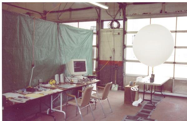
Figure 1, Balloonsonde system ready for launch, ground station and data acquisition system is on table at left.
